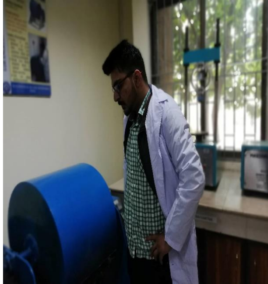
Figure 3.14 Performing Los Angeles Abrasion test
