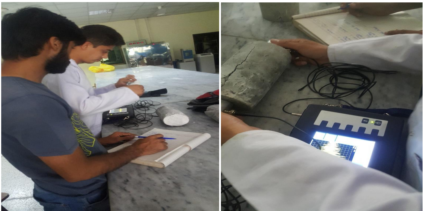
Figure 4.14 Performing UltraSonic Pulse Velocity test
