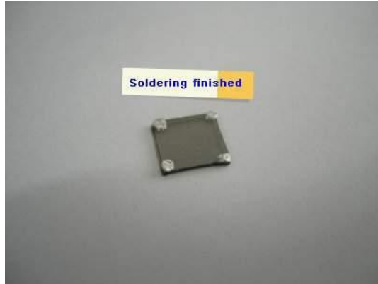
Figure 2.17: Soldered four points by use of hands
