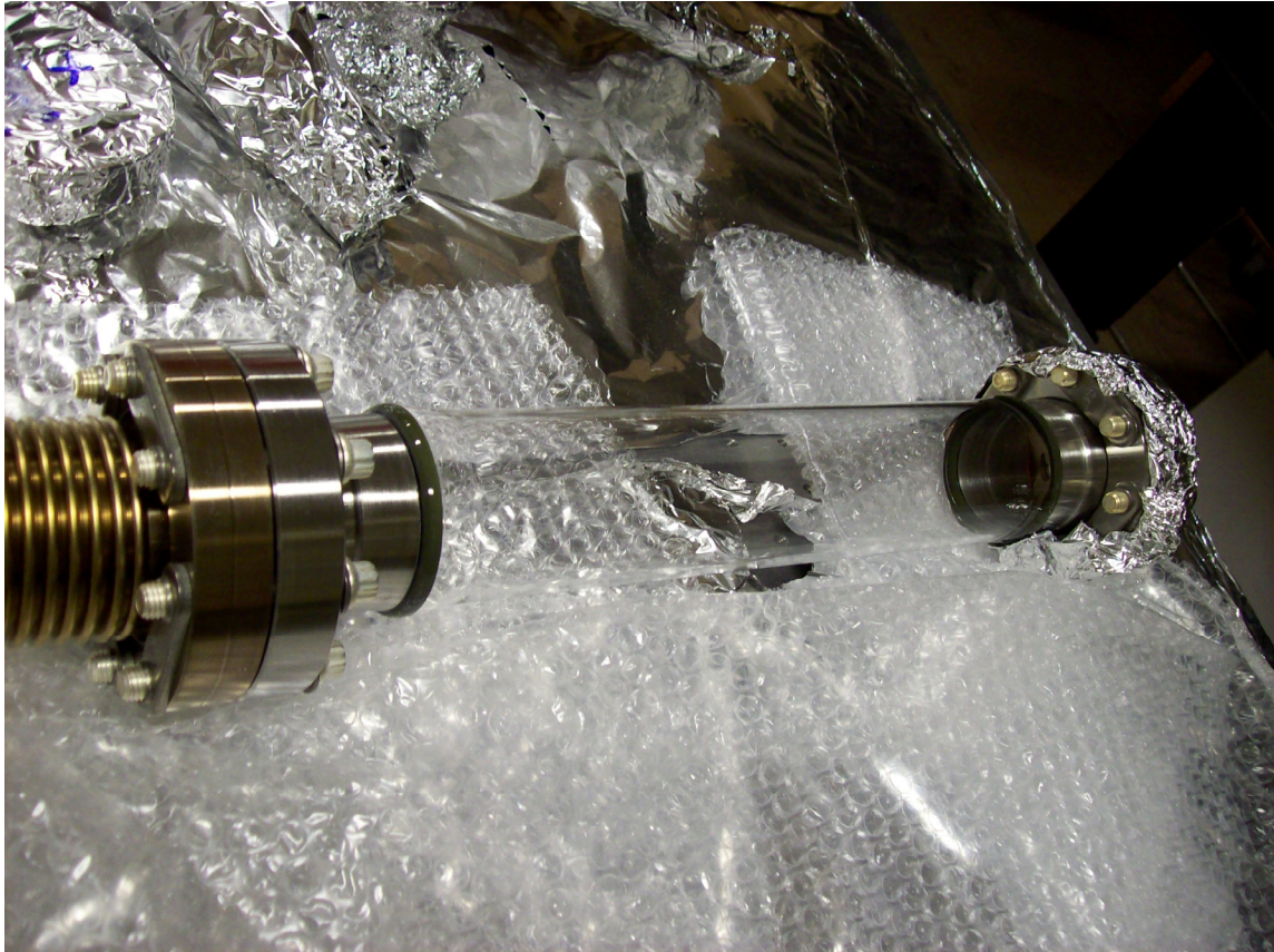
Figure 11: Vacuum Chamber used for housing \text{Rb}^{87} atoms.
