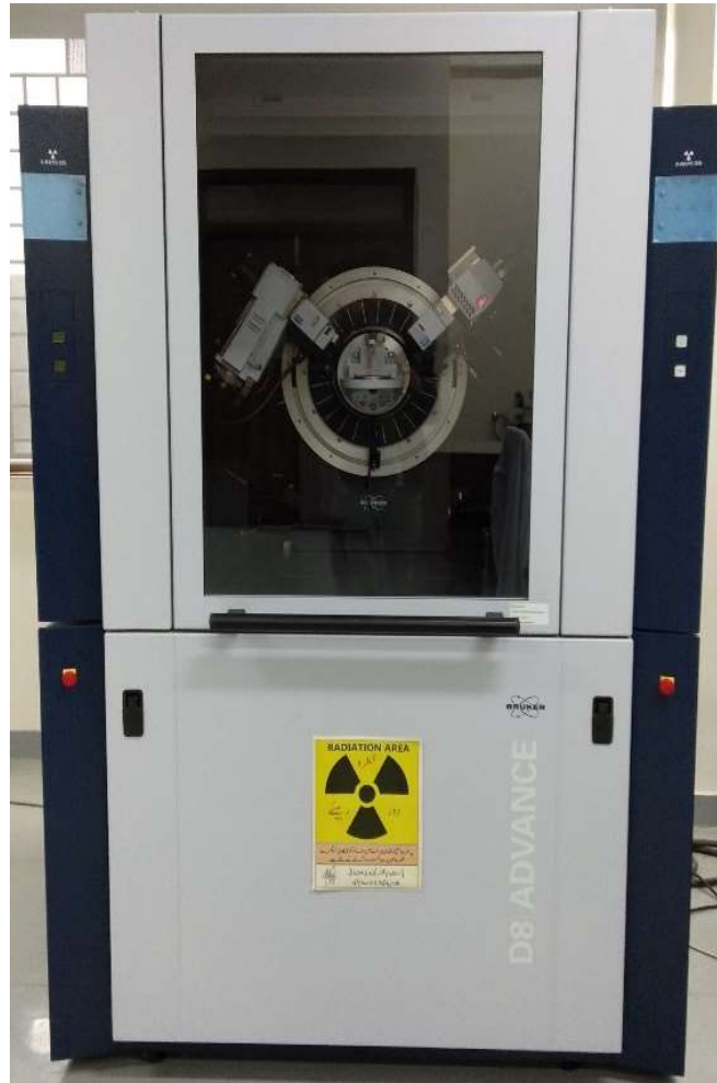
Figure 4.2 Bruker D8 advanced X-ray diffractometer
