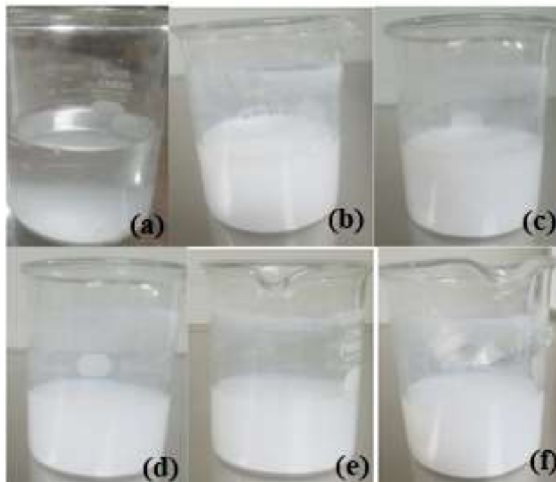
Figure 5.7 Sedimentation photograph of 0.2vol% \text{TiO}_2 - \text{H}_2\text{O} of nanofluid with surfactant (a) Before sonication (b) Day1 after sonication (c) Day17 (d) Day 32 (e) Day44 (f) Day 60
