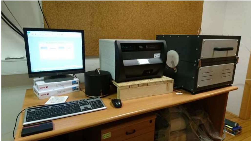
Figure 4.9 Thermal conductivity meter (Hot Disk TPS 2500s)
