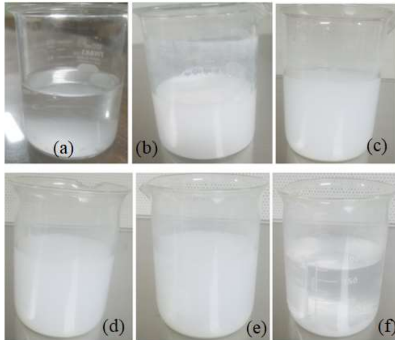
Figure 5.6 Sedimentation photograph of 0.05vol% \text{TiO}_2 - \text{H}_2\text{O} nanofluid without surfactant (a) Before sonication (b) Day1 after sonication (c) Day9 (d) Day 13 (e) Day17 (f) Day 20
