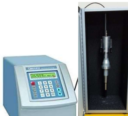
Figure 4.5 QSonica Probe Sonicator
