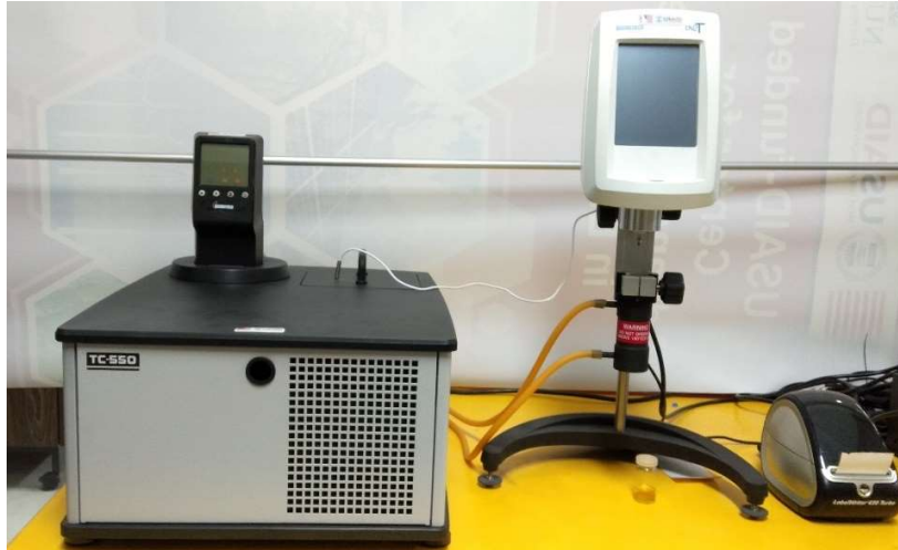
Figure 4.8 Brookfield Viscometer DV2T
