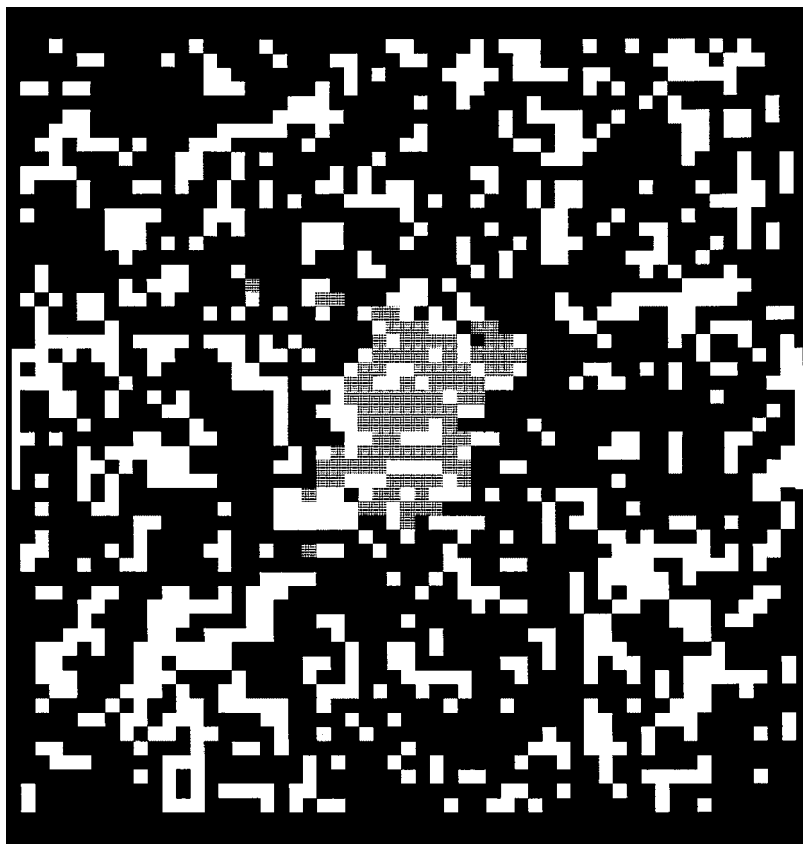
Figure 16 A model of the disruption of a crystal in water. The dark cells represent water, the white cells are cavities, and the gray cells are solute molecules.
