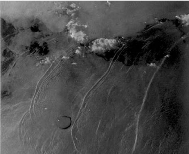
Figure 14.4 Satellite image using synthetic aperture radar (SAR) of internal wave fronts propagating westward in the South China Sea. A multiwave merger occurs in the region West of the Dong-Sha atoll, which is about 40 km in diameter. An expanded view of this nonlinear wave merger is shown in Figure 14.5. SAR images from A. Liu, private communication.
