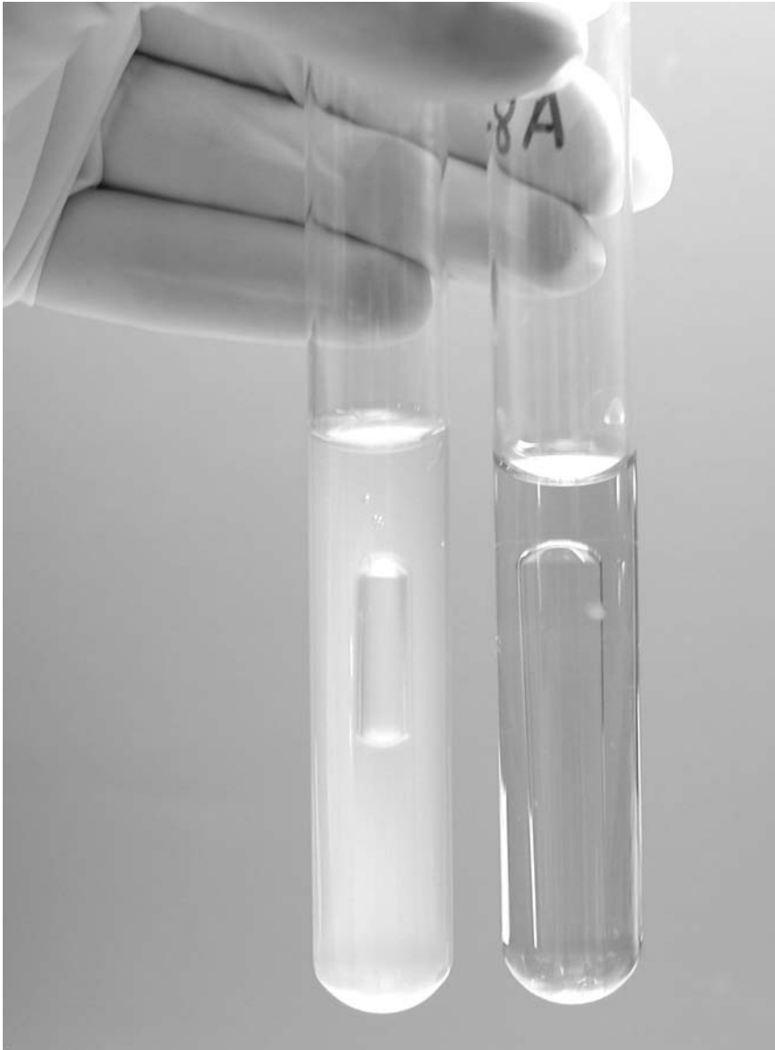
Figure 15-2 Inverted Durham tubes to collect gas. (Photo courtesy K.L. Josephson.)
