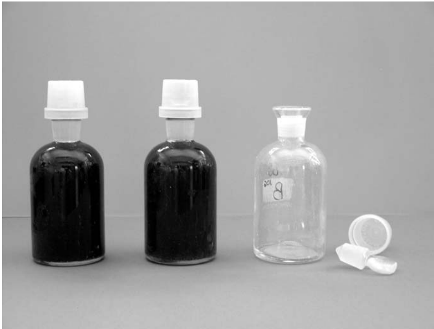
Figure 12-2 BOD bottles used for this experiment. (Photo courtesy K.L. Josephson.)
