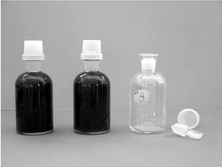
Figure 14-1 BOD bottles used in this experiment. (Photo courtesy K.L. Josephson.)
