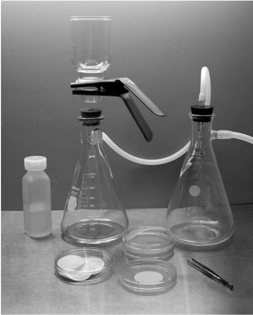
Figure 16-1 Filtration apparatus needed in this experiment. (Photo courtesy K.L. Josephson.)
