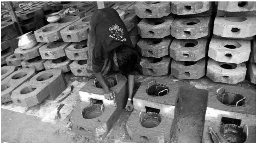
Figure 3.4 The making of a two-mouthed ICS at a GTC, Singair, Bangladesh
