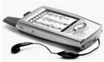
Fig 9.6 Next-generation PDA device with pen and speech based input, integral GPS and GPRS connectivity.
