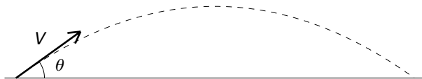
Fig. 5.10. Firing a shell at muzzle velocity V at an angle \theta to the horizontal. The shell follows a parabolic path.
