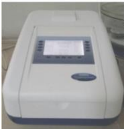
Figure 4.4: Jenway 7315 UV-Vis spectrometer present in SCME, NUST, Islamabad.
