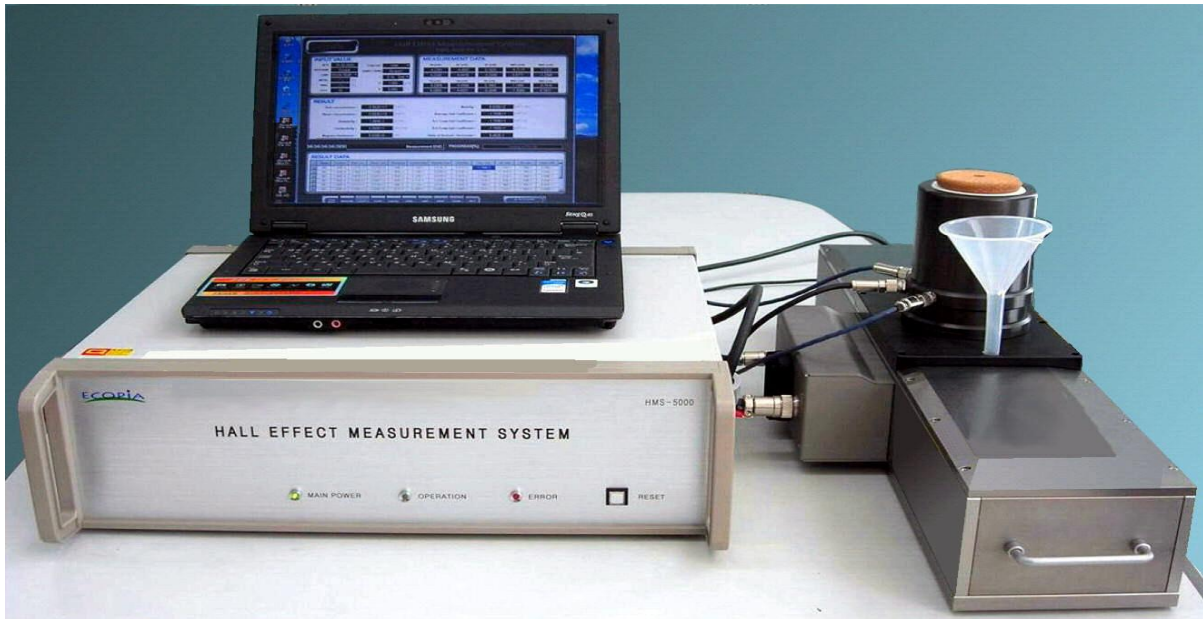
Figure 4-6: Van der Pauw HMS-5000 Variable Temperature Hall Effect Measurement System by ECOPIA [6].
