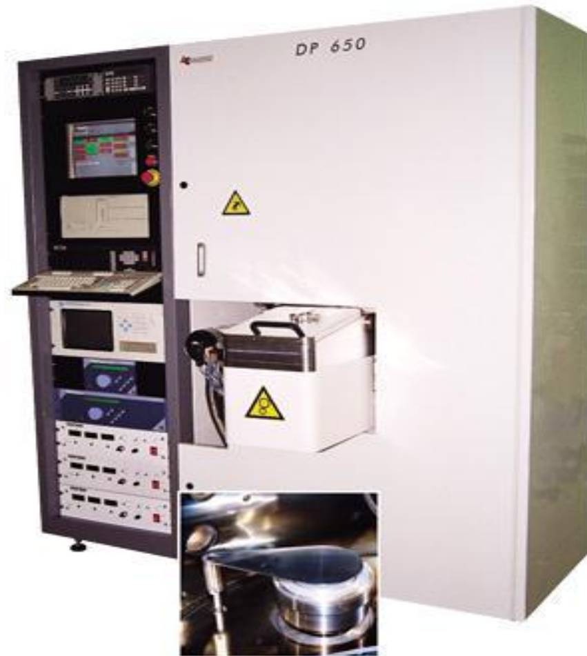
Figure 4-1: Alliance Concept DP650 RF-magnetron Sputtering System [1].
