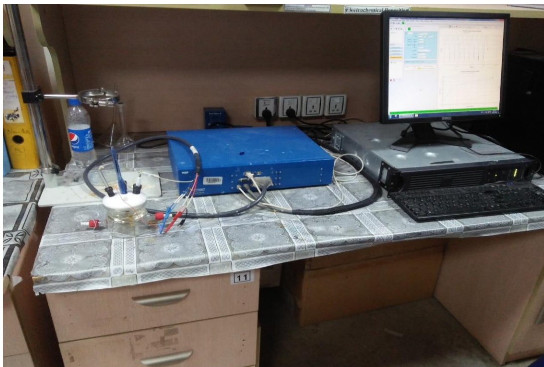
Figure 3.17 Schematic of Bio Logic VSP instrument used for electrochemical measurements.
