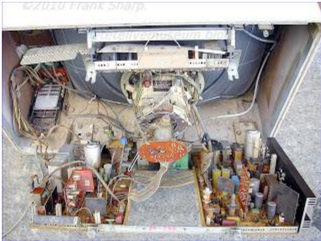
Figure 3.3. Digital TV receiver contains Mn-ferrites deflection yokes [17]
