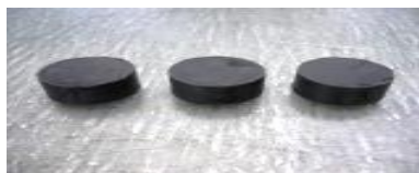
Fig 3.3 Compression set samples
