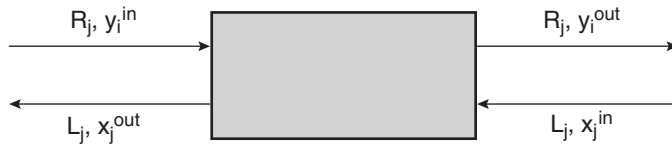
Figure 10.3-13 Mass balance diagram for mass exchange network synthesis
