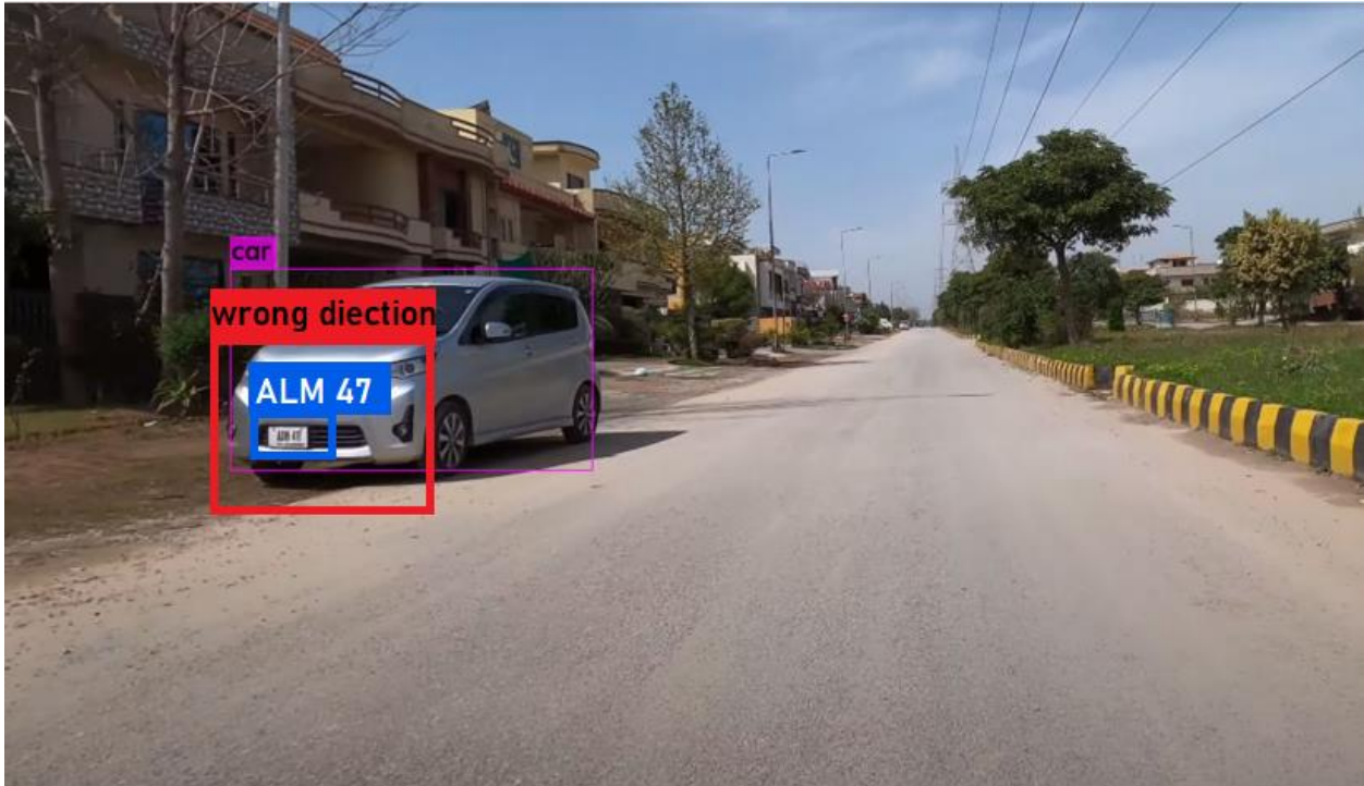
Figure 3.5.1: Wrong direction detection result
