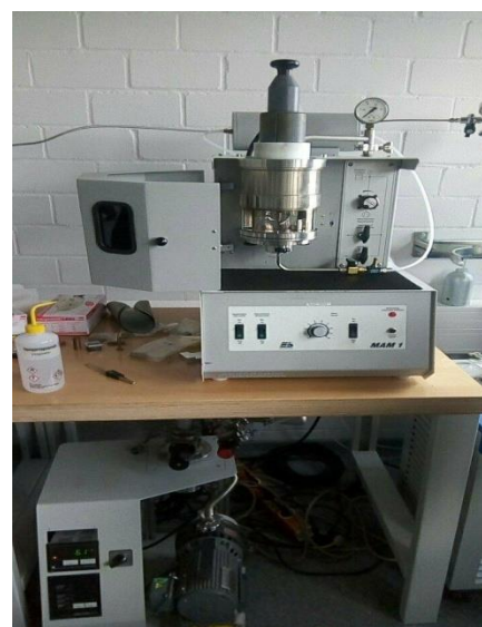
Figure 21 Arc Melt Furnace
