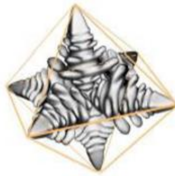
Figure 42 Schematic representation of an octahedral crystal growing through the liquid sample. The blue area shows the intersection of the crystal with the sample surface. The light gray body is the part of the crystal that solidifies below the surface.
