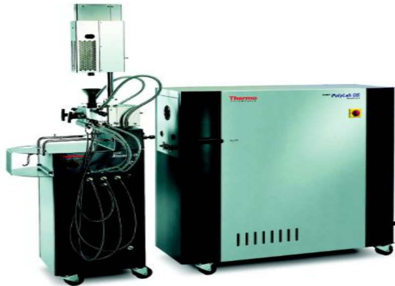
Figure 3: HAAKE Poly Lab OS internal engineering mixer system.
