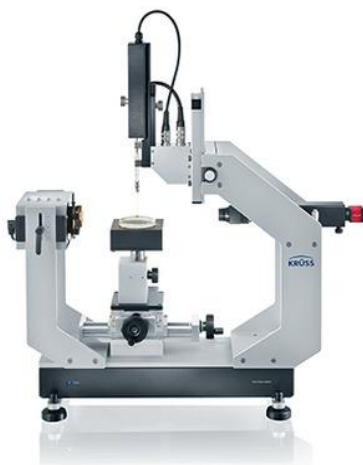
Fig 3.3.3 Drop Shape Analyzer – DSA30 (Krüss) at SCME NUST
