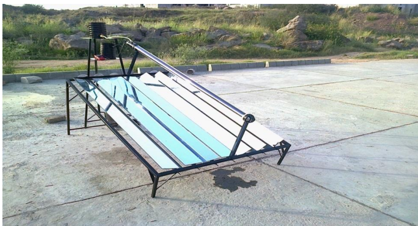
Figure 5: photograph of Solar Concentrator with Fresnel Mirrors
