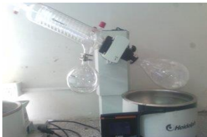
Figure 3.2 Drying in rotary evaporator
