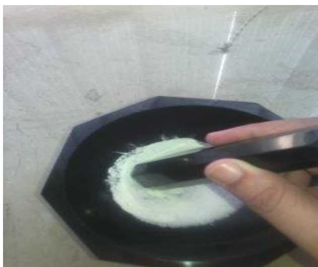
Figure 3.3 Mixing and grinding Urea and nano powder of titania
