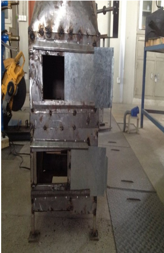
Figure 13 Fuel Charging door and Furnace Cleaning Door
