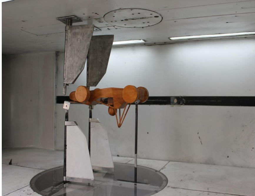
Figure 4-19: wind tunnel “inverted with dummies” analysis
