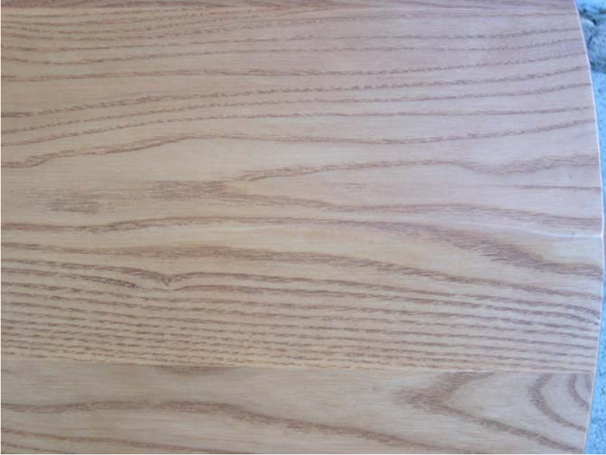
Figure 1.2. Wood is a very good example of a porous medium which exhibits a strong anisotropy. The grain effect is clearly visible here. This is a material which is approximately transversely isotropic
