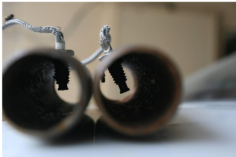
Figure 5.2.2 - Thermocouple in Pipe (1)
