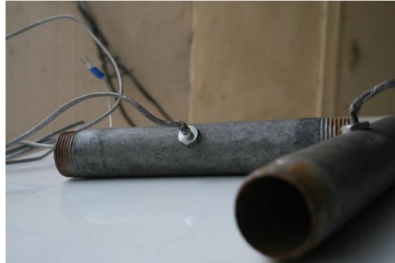
Figure 5.2.3 - Thermocouple in Pipe (2)
