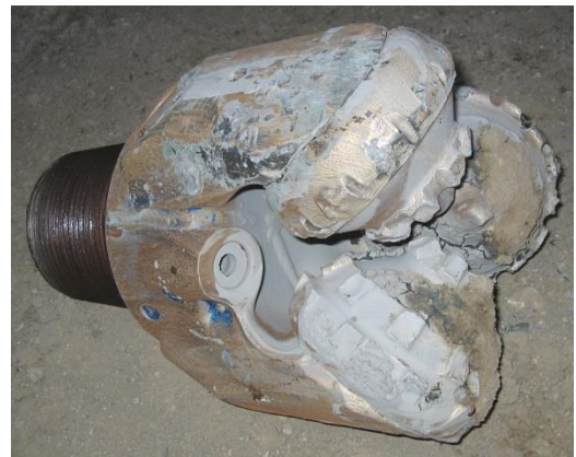
Figure 2 Worn Tricon Drill Bit
