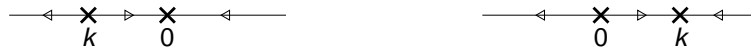
Fig. 8.1. The phase diagram for the equation \dot{x} = kx - x^2 , for k < 0 (left) and for k > 0 (right).
