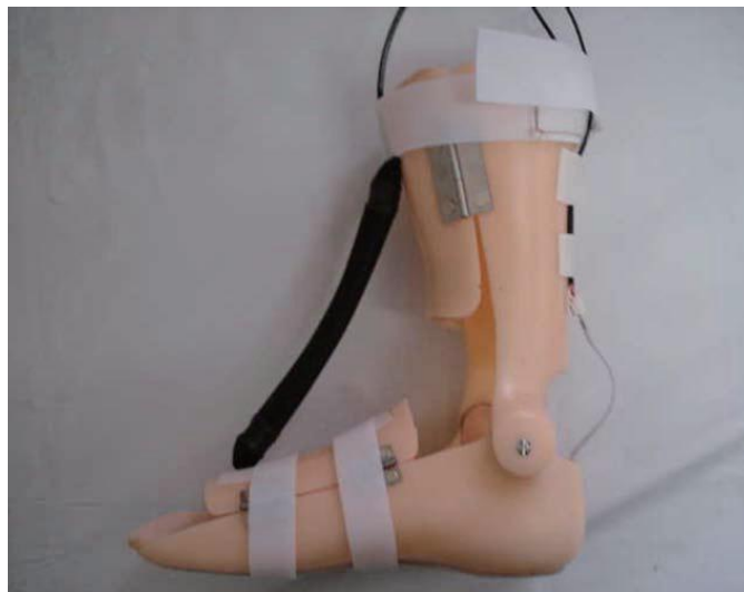
Figure 2: Ankle foot Orthosis by the use of Pnuematic Muscles
