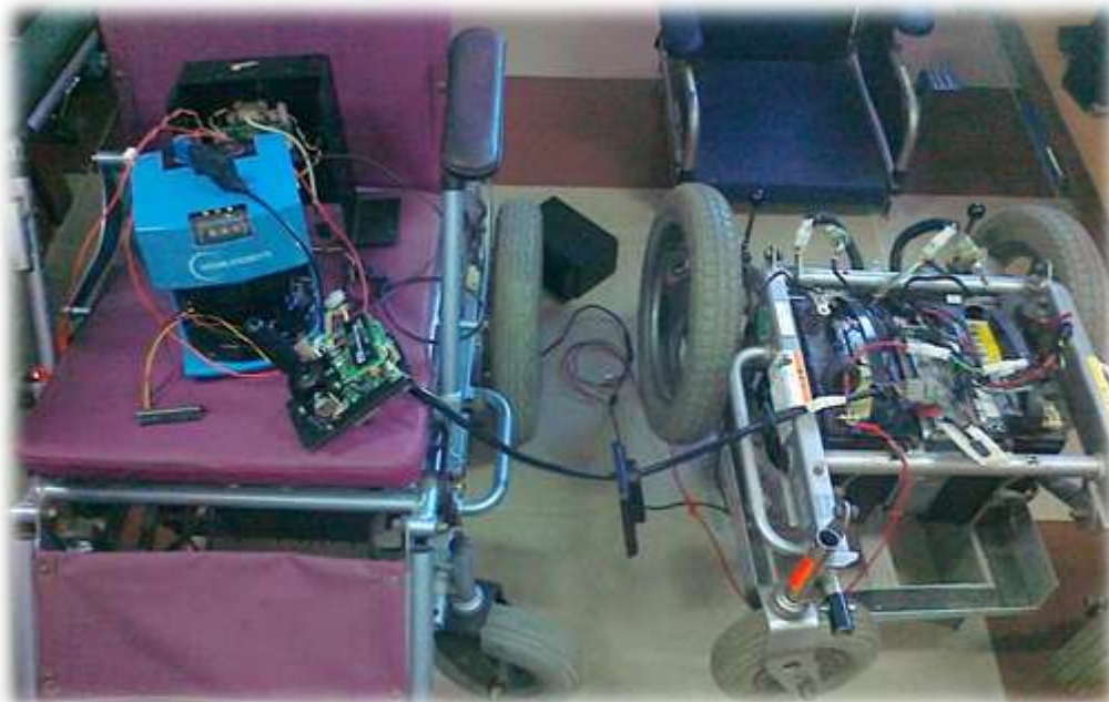
Fig 15: Shifting control form joystick to LabView
