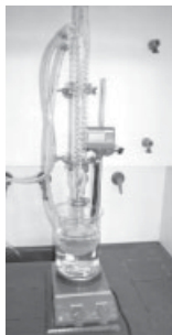
Figure 5.40 Maceration mini-plant equipment [10].
