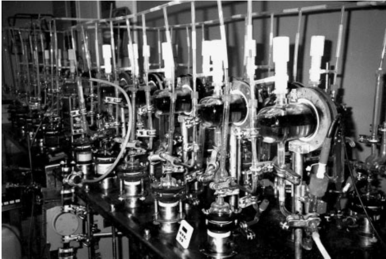
Figure 5.36 Mixer-settler battery with 10 stages laboratory scale i.d. 50 mm (Bayer Technology Services GmbH).
