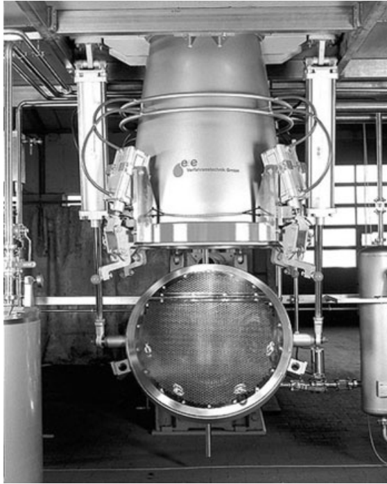
Figure 6.20 Percolation extractor 1 m 3 ; (Courtesy of e&e Verfahrenstechnik GmbH) [35].
