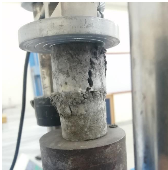
Figure 3.9: Failed UCS Sample
