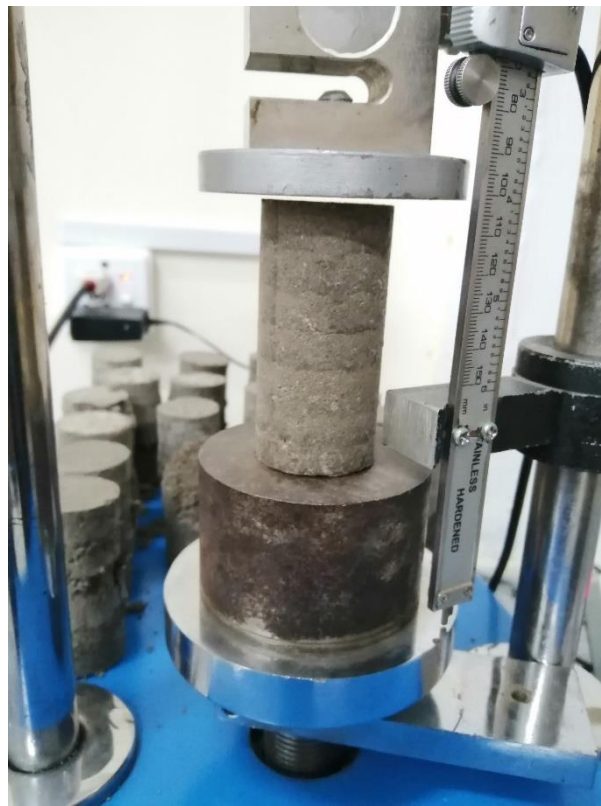
Figure 3.8: UCS Test Sample placed in Compression Testing Machine
