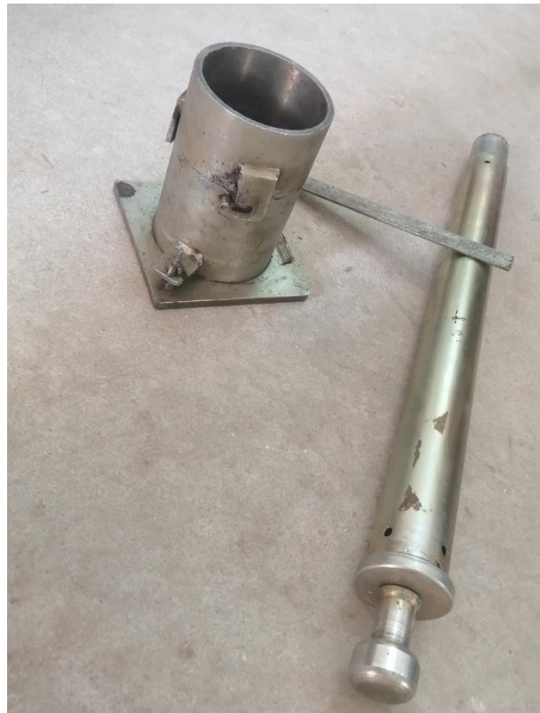
Figure 3.7: Compaction Test Assembly
