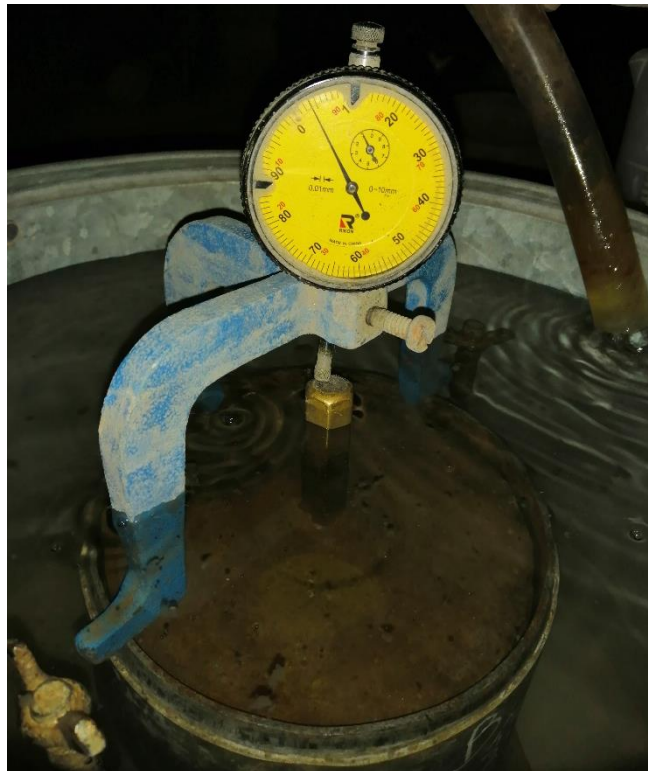
Figure 3.10: Soaked CBR Sample Assembly
