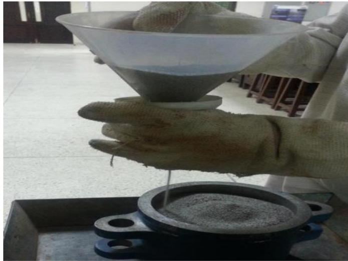
Figure 3.9: Pictorial view of the arrangement of equipment for the determination of  $e_{\max}$  and  $e_{\min}$ .
