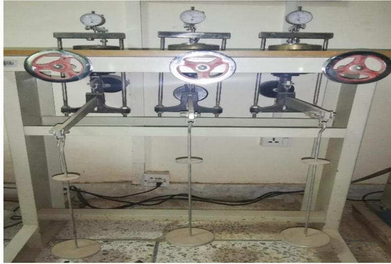
Figure 3.8: Odometer machine for swelling test
