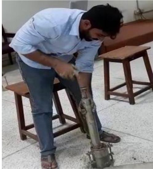
Figure 3.4: Compaction test performed in the laboratory
