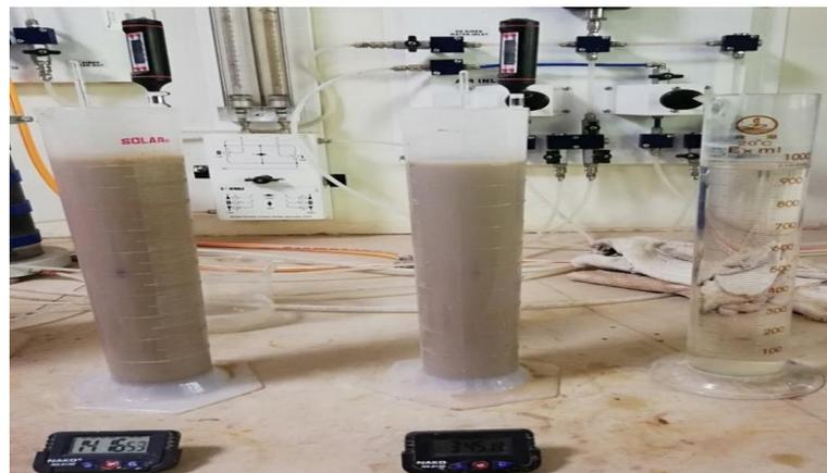
Figure 3.2: Scheme of the hydrometer analysis in the laboratory
