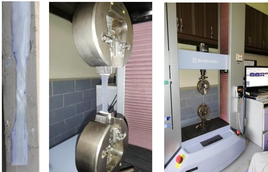
Figure 3.10: Pictorial views of the specimen preparation and arrangement of the tensile test of the polythene sheet
