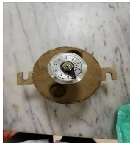
Figure 3.6: Portable vane shear test
