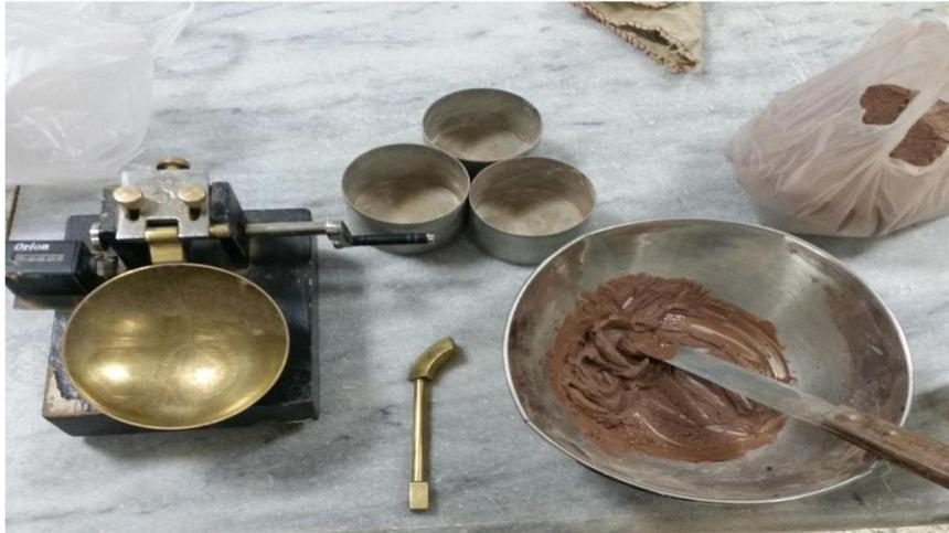
Figure 3.3: Liquid limit test arrangement in the laboratory
