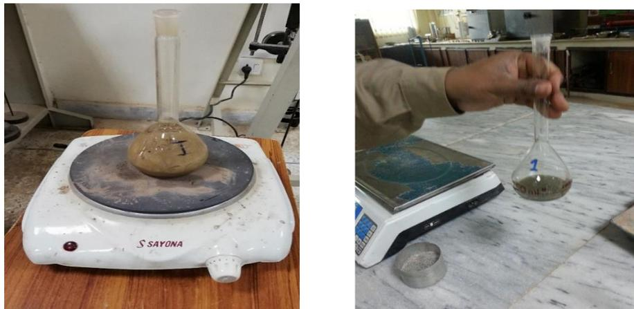
Figure 3.7: Pictorial views of specific gravity tests
