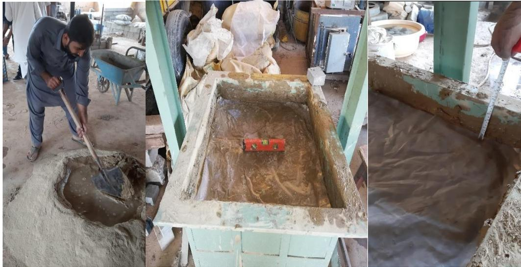
Figure 3.14: View of soft clay preparation and layout of the polythene sheet
