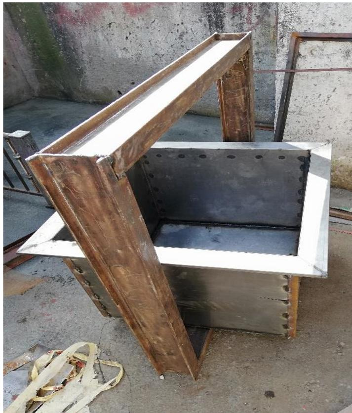
Figure 3.11: View of small-scale loading beam and steel box
