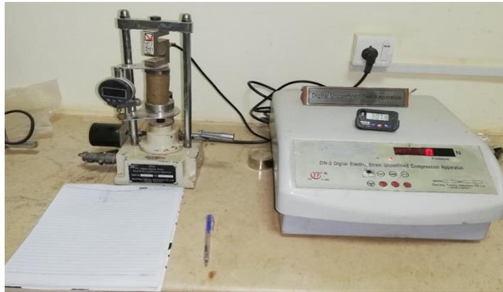
Figure 3.5: Scheme of unconfined compressive strength test
