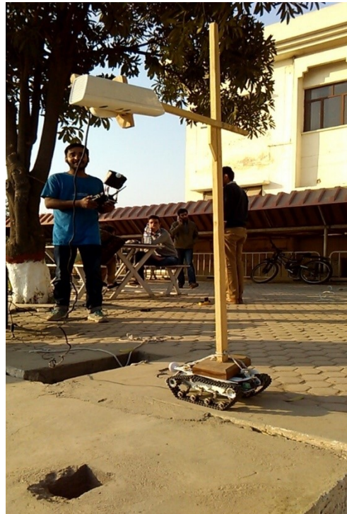
Figure 4.1: Test Rig with Kinect and accelerometer are mounted on UGV for Experimentation
