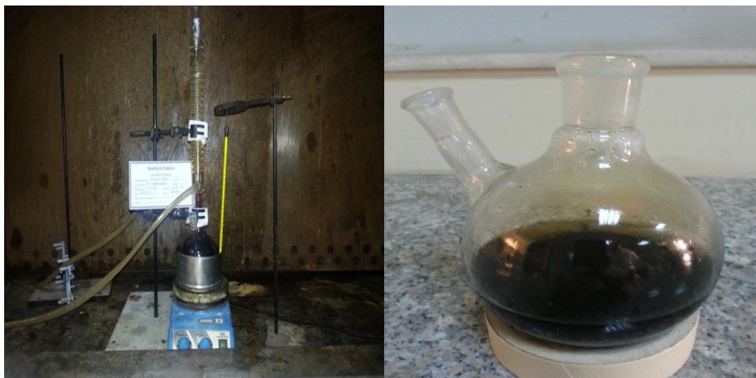
Figure 3.3: Images of reflux process (left) and solution after reflux (right).
