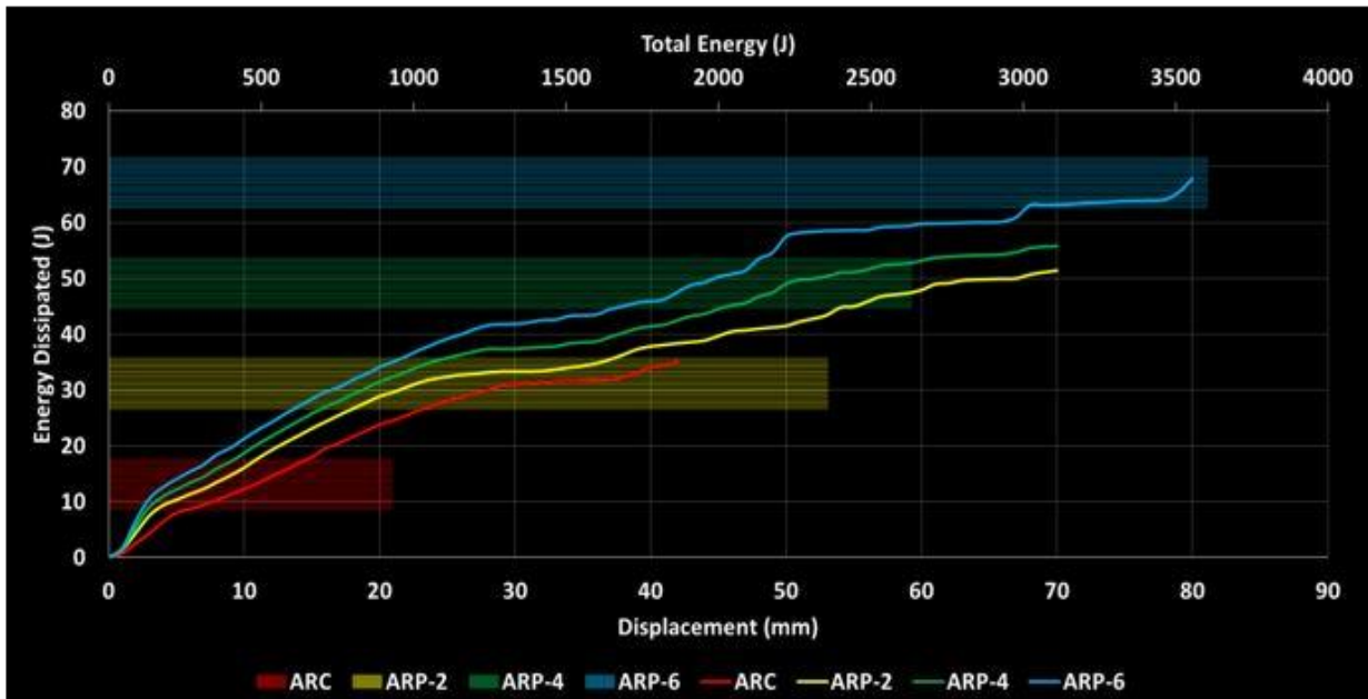
Figure 8: Comparison of 1:1.5:3 Mix Ratio, Reinforced Slabs (lines show energy dissipation)
