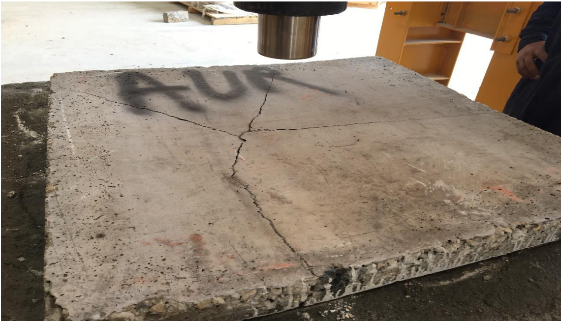
Figure 29 Cracking Pattern of Unreinforced Slab
