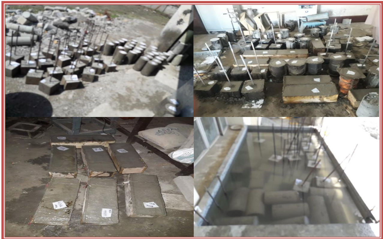
Figure 8 Casting of Concrete Sample
