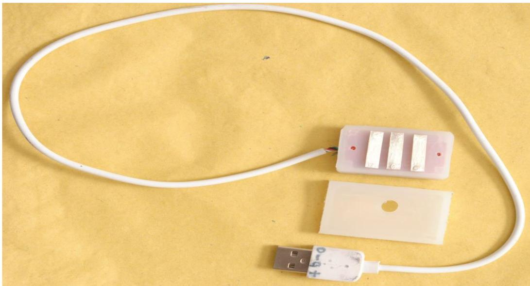
**Figure 4.14** Silver electrodes attached directly to Pre-amplifier of SEMG sensor
