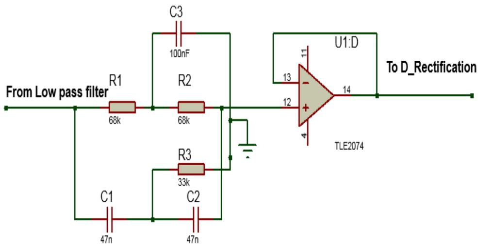
**Figure 4.4** Twin T notch filter used in sensor fabrication.
