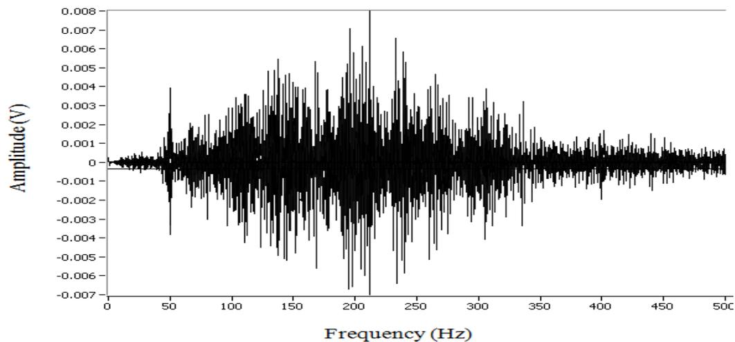
**Figure. 5.7** FFT of filtered SEMG signal is acquired from fabricated sensor through Labview software. Filtration of raw SEMG signal is carried out through high, low and notch filters of fabricated SEMG sensor.
