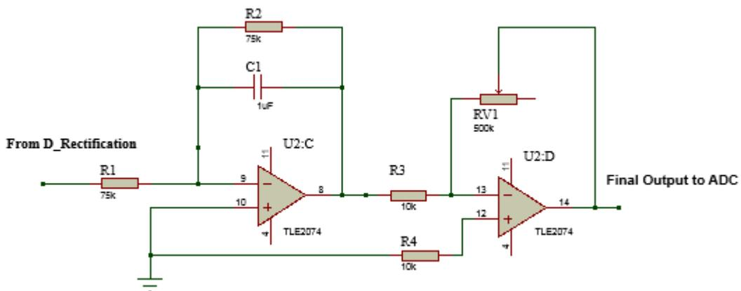
**Figure 4.6** Smoothing of EMG signal at 2.13 Hz.
