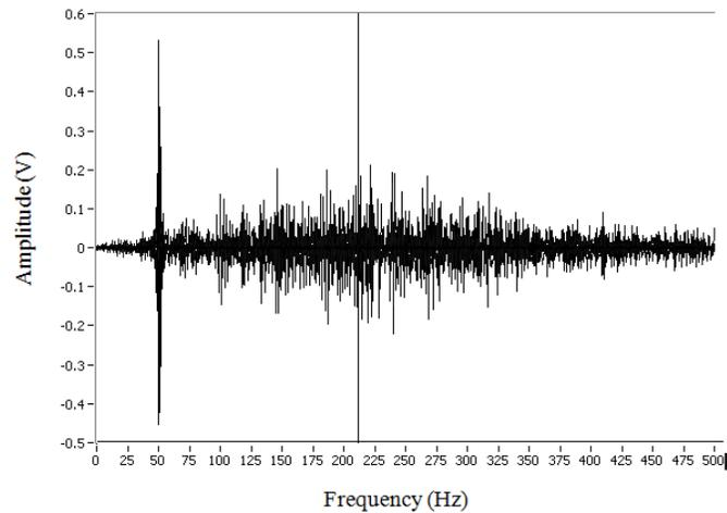
**Figure 1.12** Spectrum of raw EMG signal
