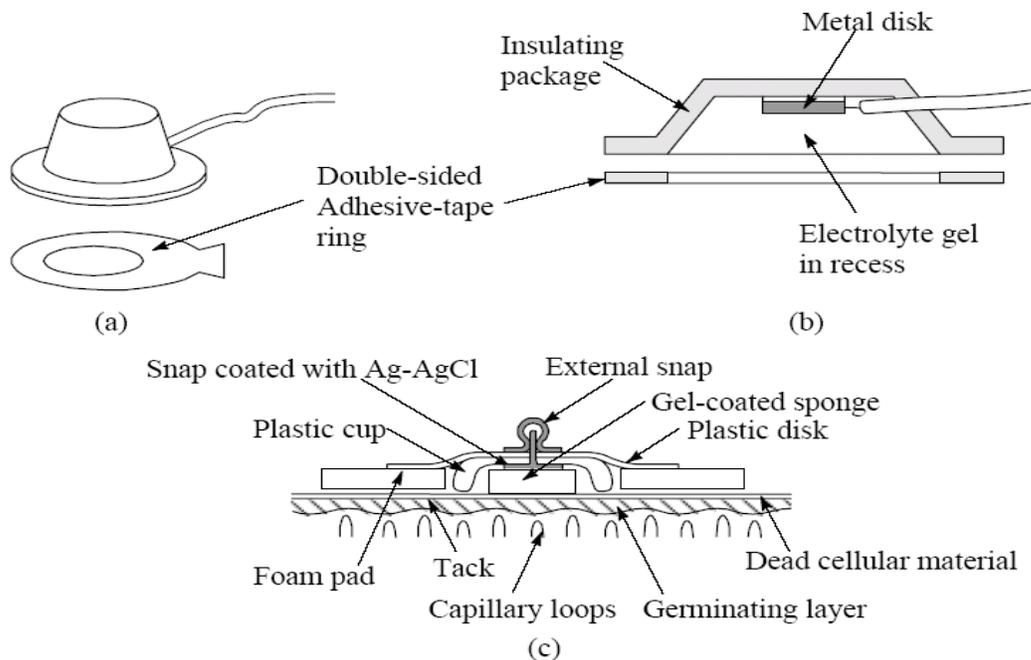
**Figure 1.17:** a) Floating electrode, b) Cross-sectional view, c) Disposable Electrode [14]
