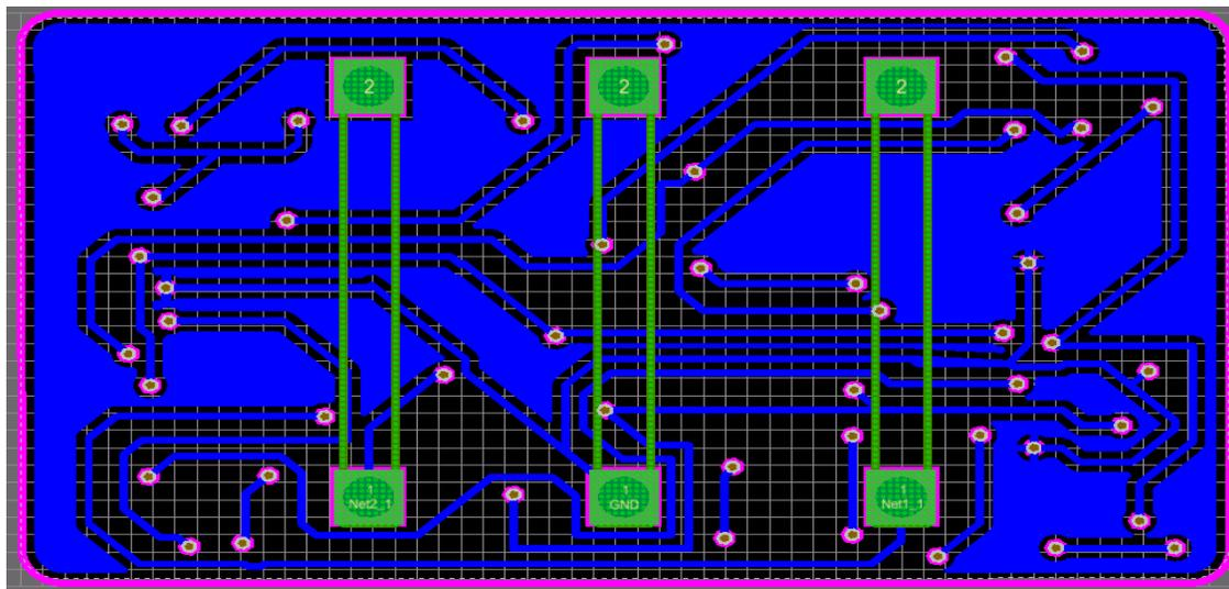
**Figure 4.11** Bottom view of PCB of SEMG sensor
