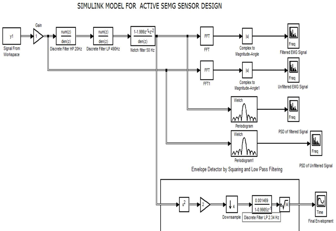
**Figure 4.7** Matlab Simulink model for designing SEMG sensor.
