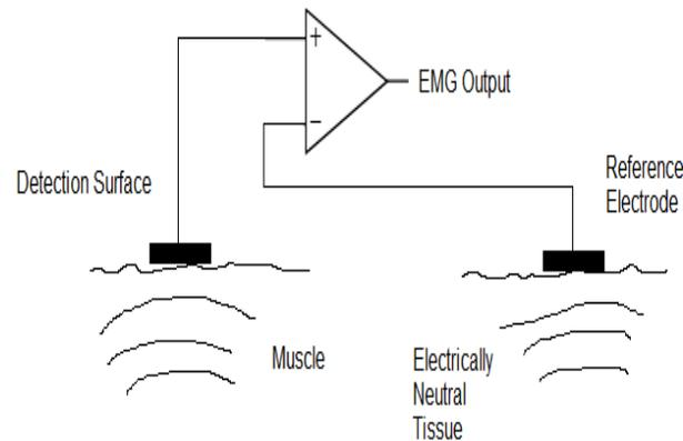
**Figure 3.8** Monopolar signal acquisition technique
