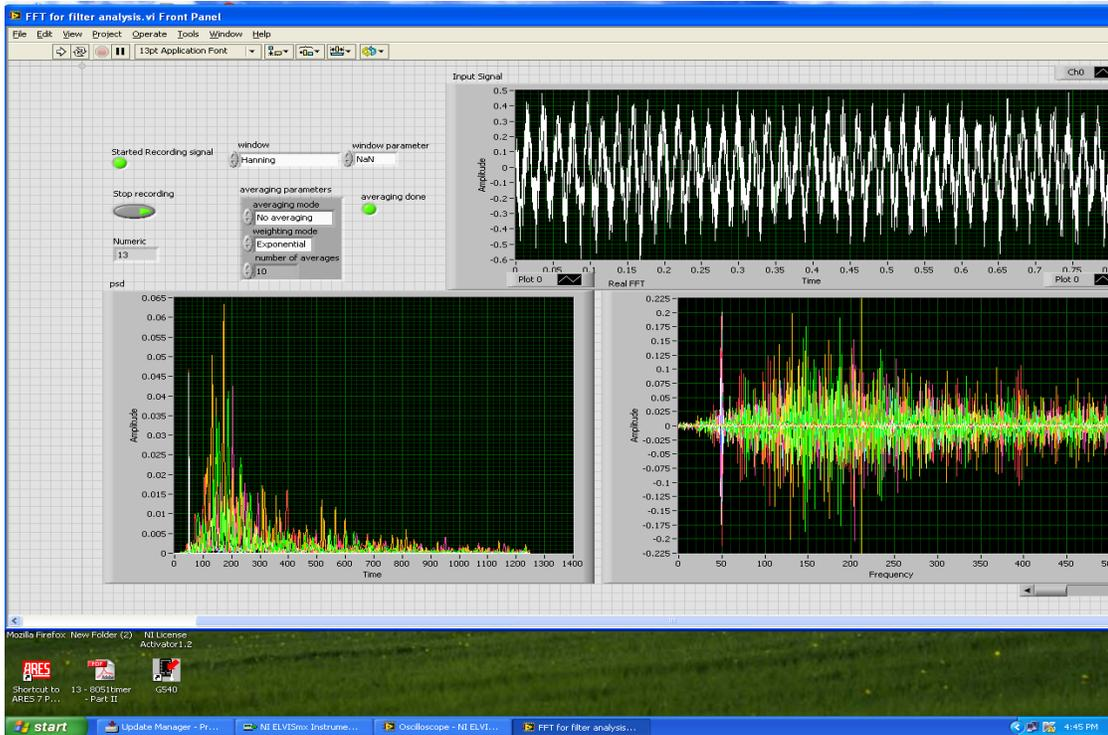
**Figure 4.16** FFT and PSD of raw SEMG signal acquired from developed sensor
