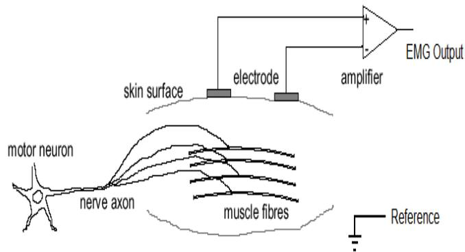
**Figure 3.9** Bipolar signal acquisition technique
