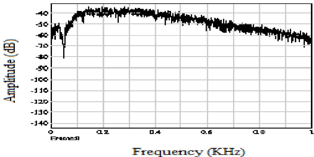
**Figure. 5.3** PSD of filtered EMG signal is acquired from this simulink model by using Hanning window in Periodogram block.
