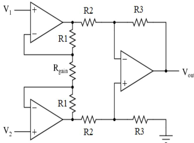
**Figure 3.7** Three amplifier instrumentation amplifier
