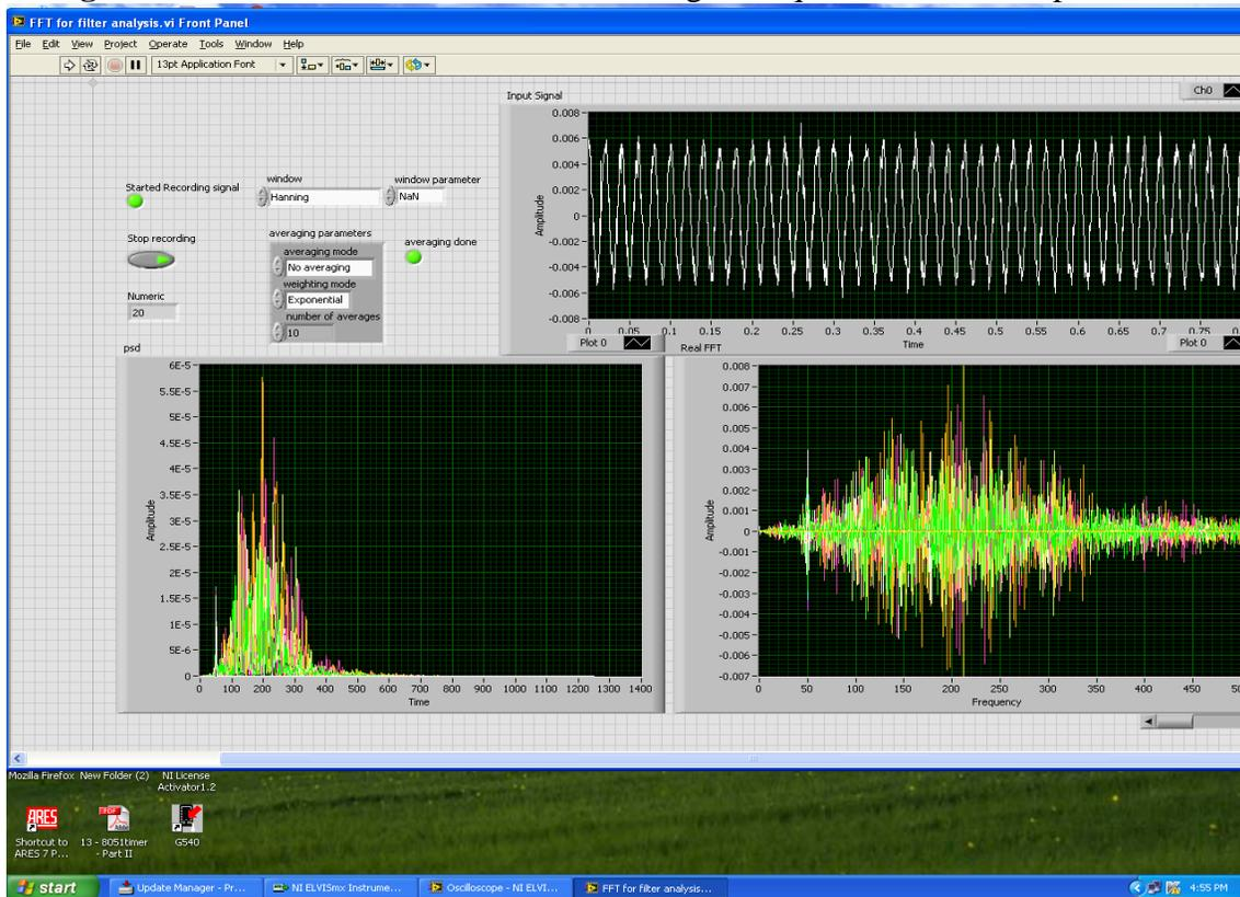
**Figure 4.17** FFT and PSD of conditioned signal acquired from developed sensor
