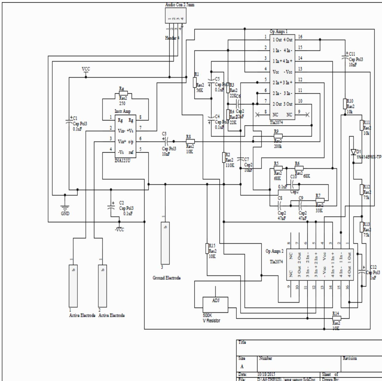
**Figure 4.9** Schematic of the developed sensor
