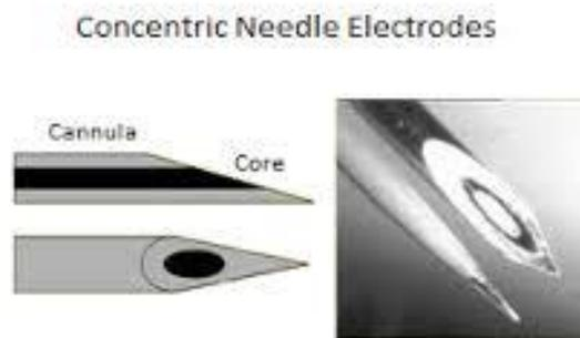
**Figure1.15** Concentric needle electrode [12]
