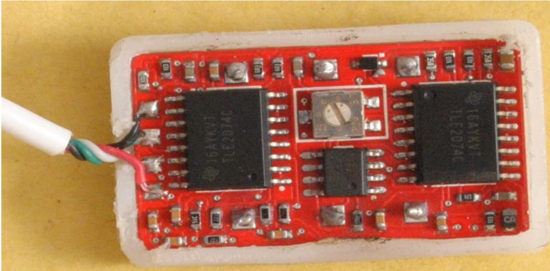
**Figure 4.15** Top view of the developed active SEMG sensor.
