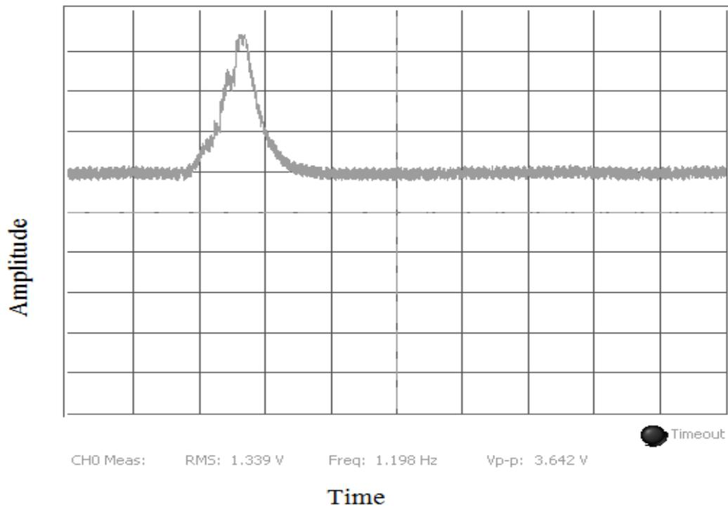
**Figure. 5.9** Envelopment of SEMG signal acquired from fabricated sensor.
