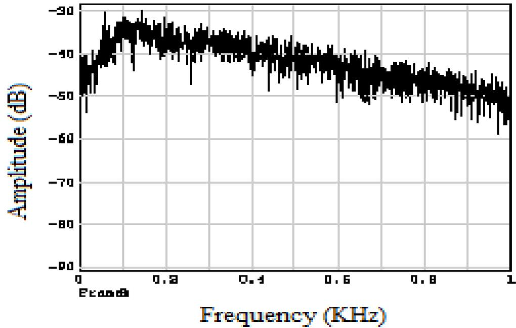
**Figure. 5.4** PSD of unfiltered EMG signal is acquired from simulink model by using Hanning window in Periodogram block.
