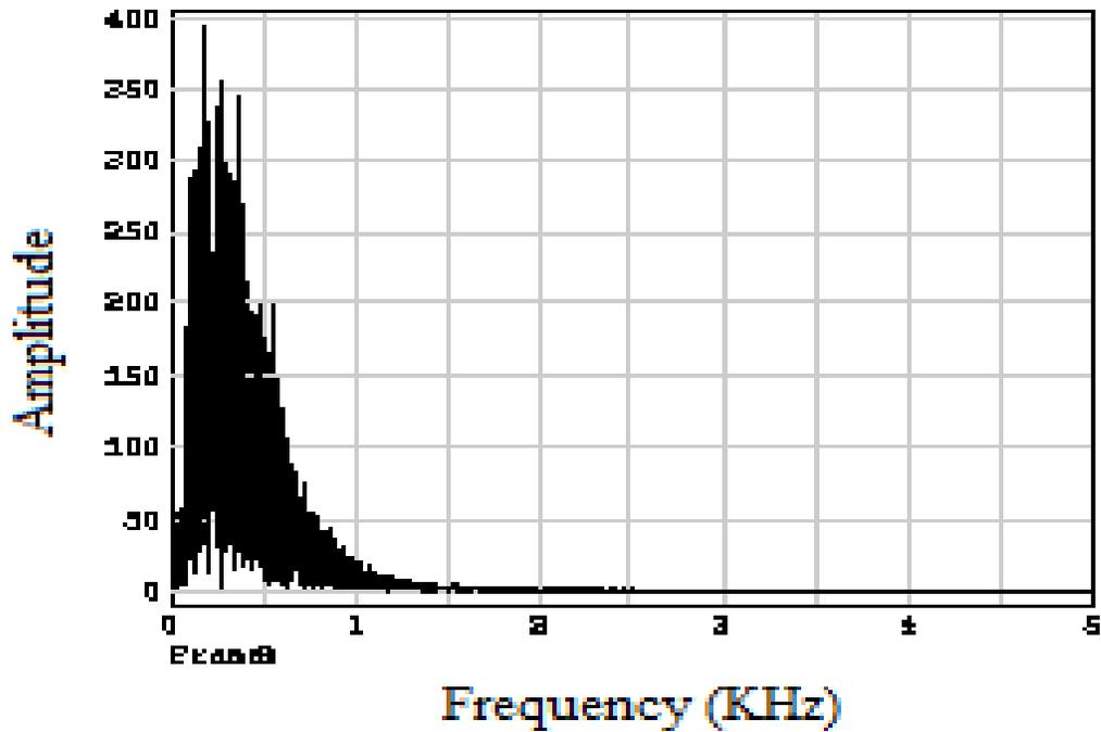
**Figure 5.2** Spectrum response of filtered EMG signal against 2<sup>nd</sup> order high pass filter ( $f_c=20\text{Hz}$ ) and low pass filter ( $f_c=490\text{Hz}$ )
