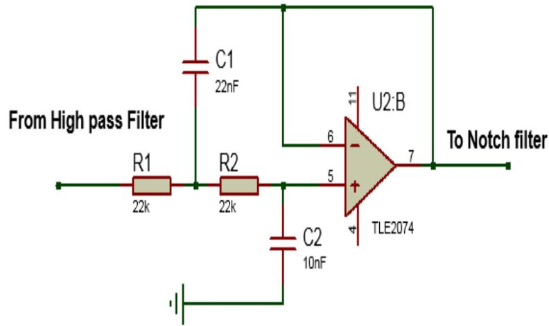
**Figure 4.3** Low pass filter at the slope rate of -12dB/octave.
