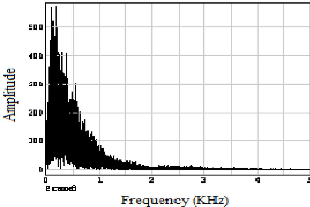
**Figure 5.1** FFT Spectrum of raw EMG signal (Amplitude Vs Frequency (KHz)) is acquired from the Simulink model. This spectrum shows that EMG signal contains both intrinsic/extrinsic noises.
