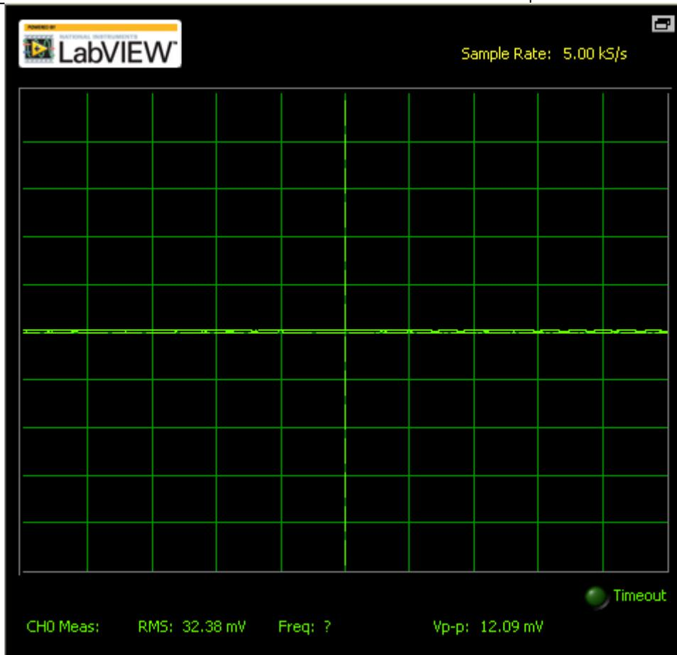
**Figure. 5.10** Relax muscle response acquired from fabricated sensor.
