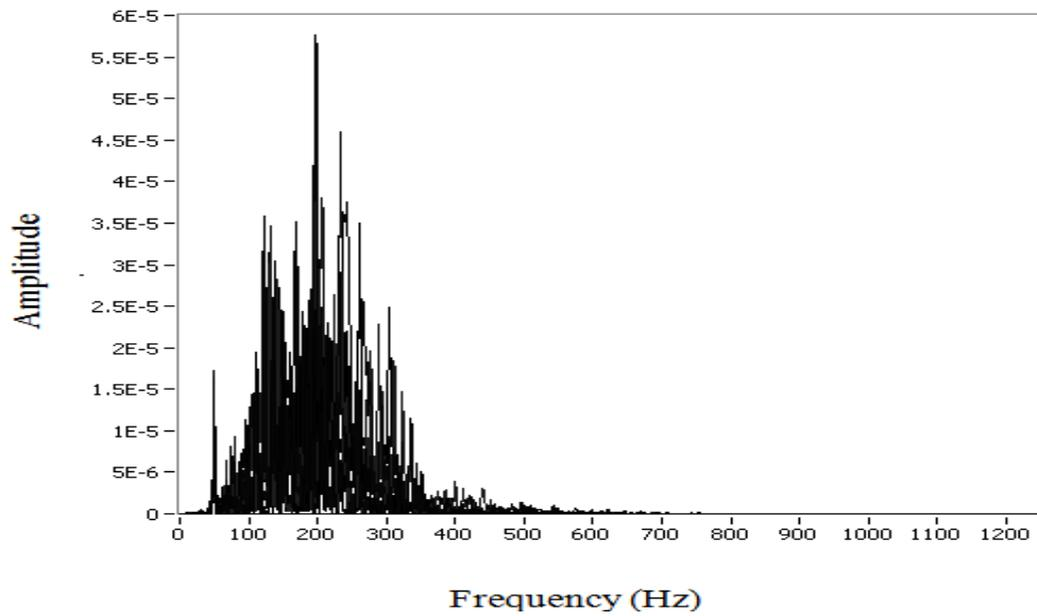
**Figure. 5.8** PSD of SEMG signal is acquired from fabricated sensor through Labview software.
