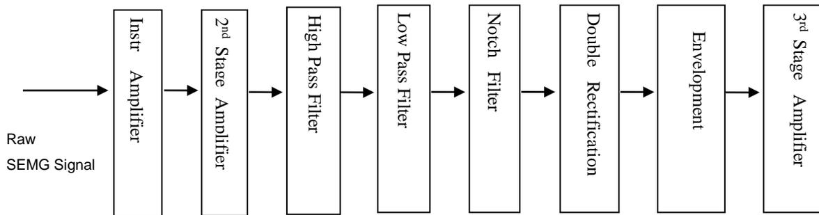
**Figure 4.8** Block diagram for development of active SEMG sensor
