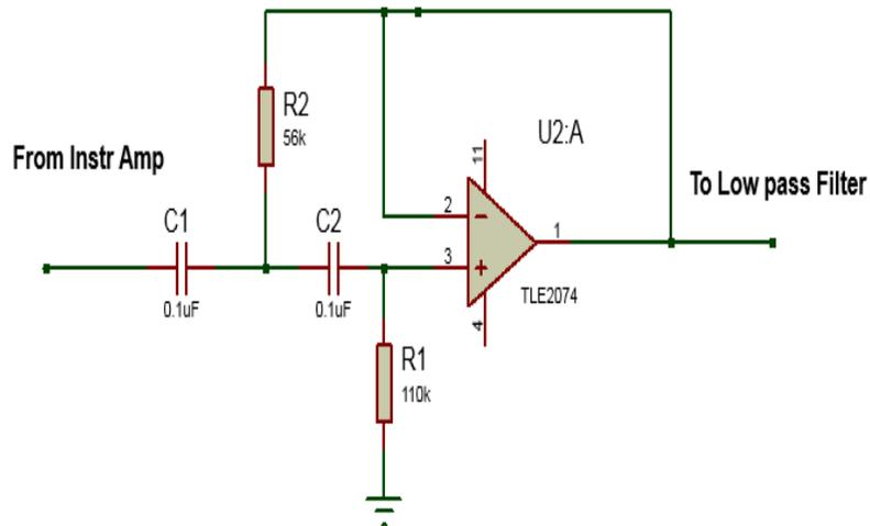
**Figure 4.2** High pass filter at the slope rate of -12dB/octave.
