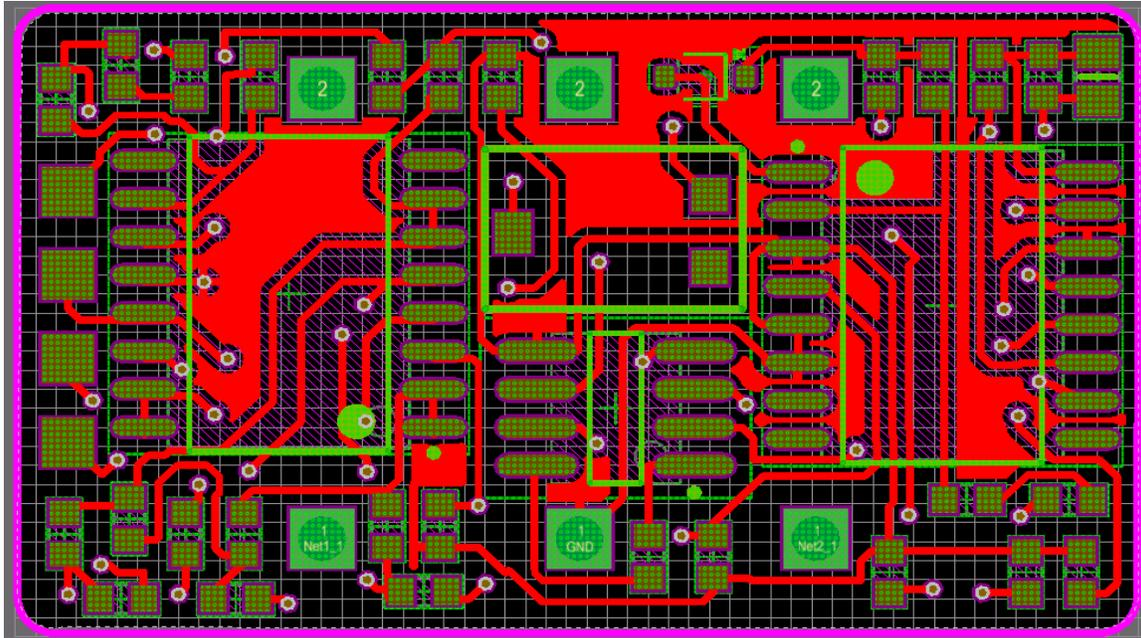
**Figure 4.10** Top view of PCB of SEMG sensor
