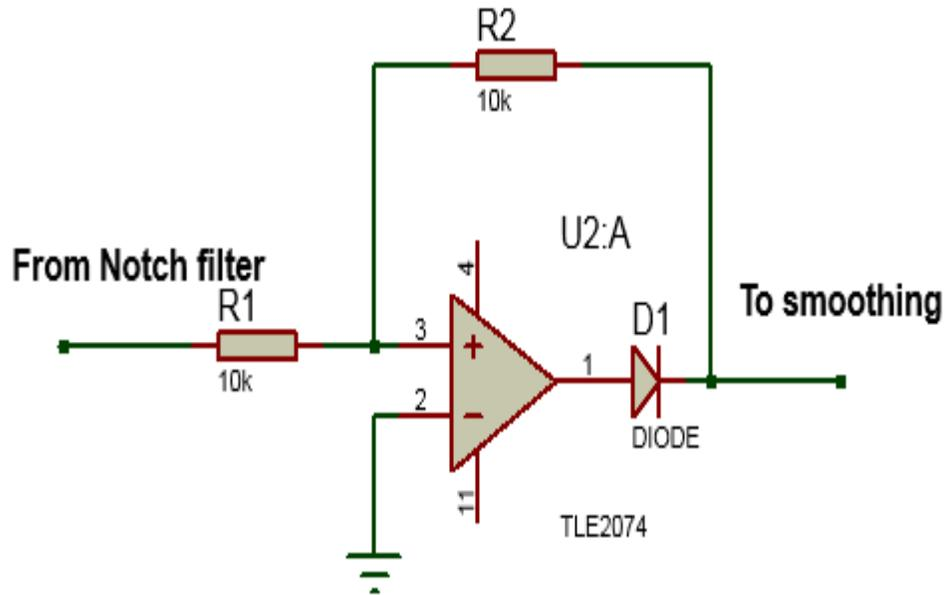
**Figure 4.5** Double rectification circuit used in sensor fabrication.
