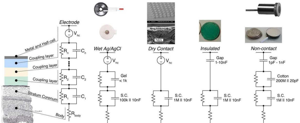
**Figure 3.4** Skin-electrode impedance against different surface electrodes
