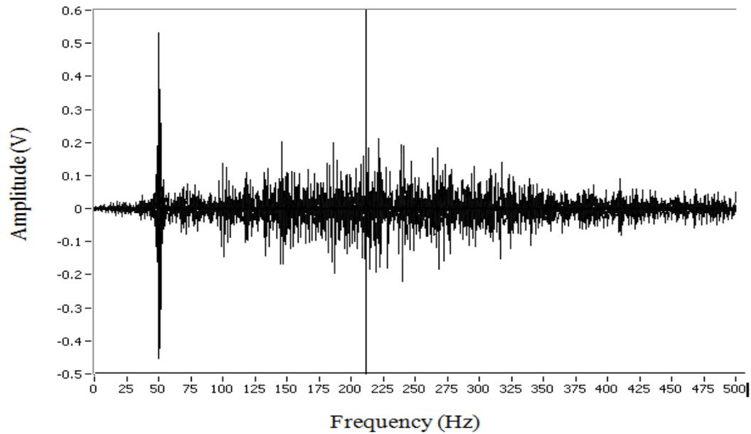
**Figure. 5.6** FFT of Raw SEMG signal acquired from fabricated sensor.
