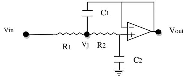
**Figure 4.1** 2<sup>nd</sup> order Sallen key low pass filter
