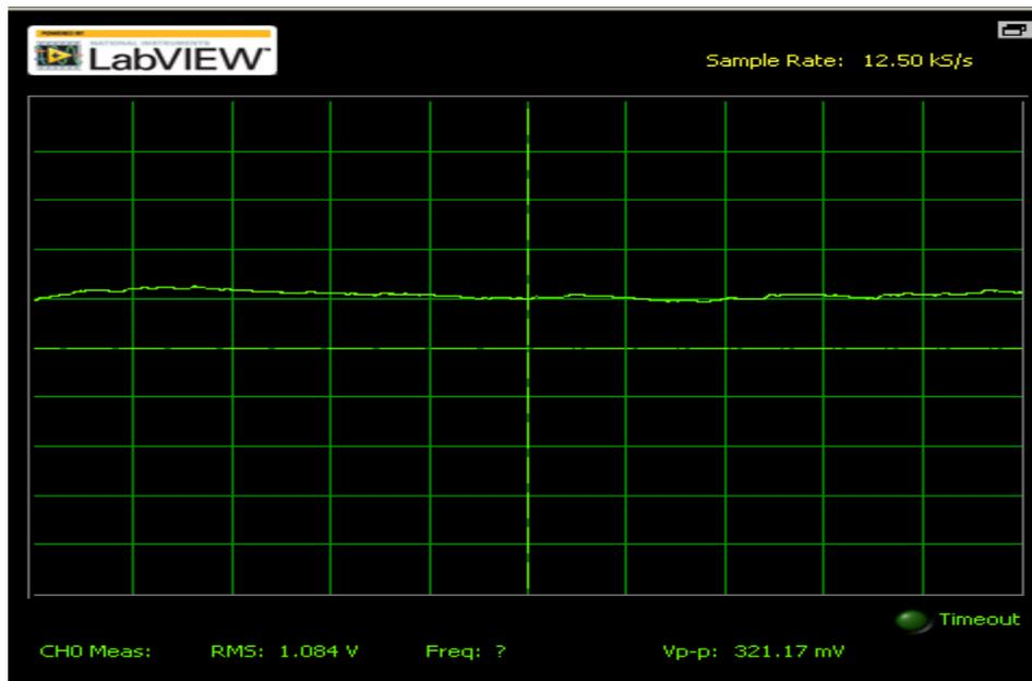
**Figure. 5.12** Prolonged muscle response after 1 min and 25 sec acquired from fabricated sensor.
