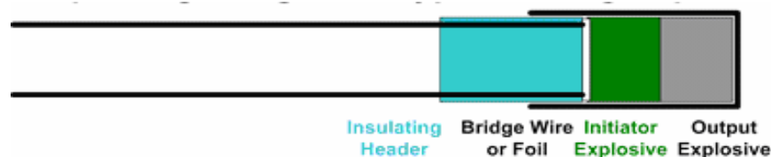
Figure 1.4 Flushed bridge detonator
