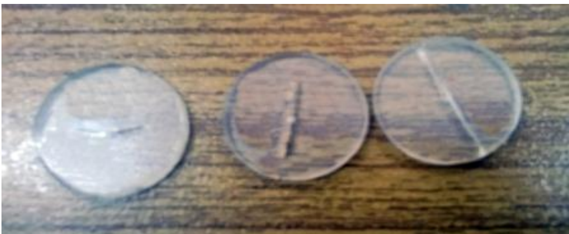
Figure 21: Indentation in Plexiglas with the conical indenter showing well defined radial cracks
