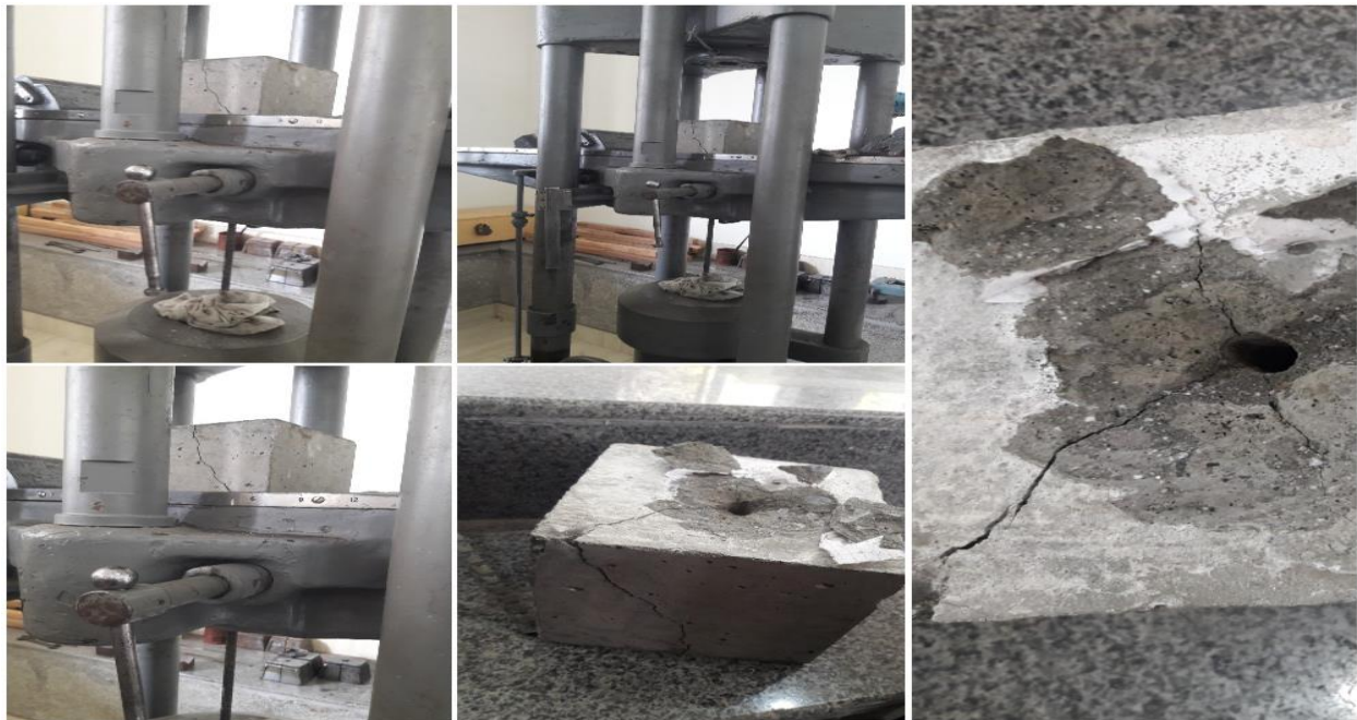
Figure 7 pull out test setup
