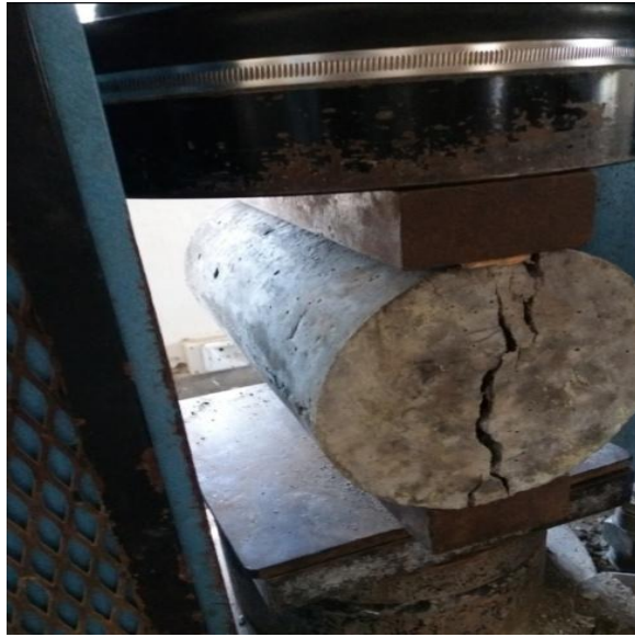
Figure 3.9: Testing of cylinder for split tensile strength
