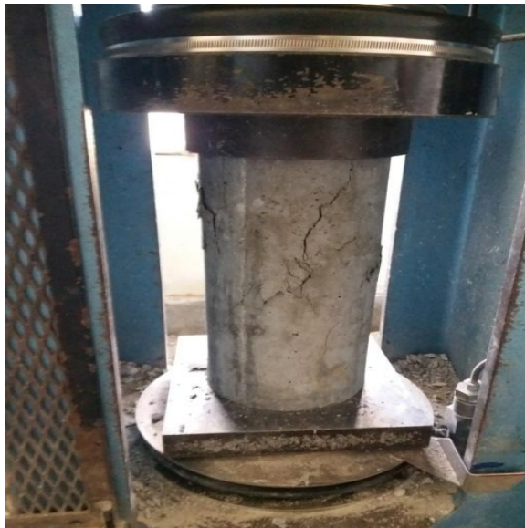
Figure 3.8: Testing of cylinder for compressive strength
