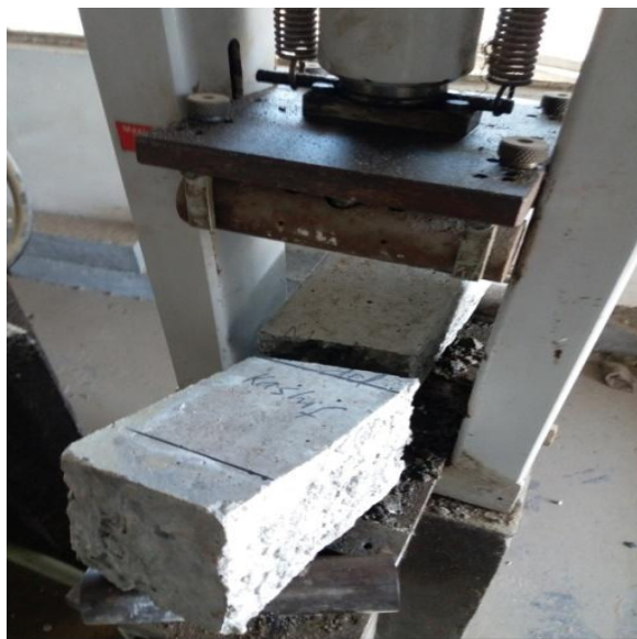
Figure 3.10: Testing of beam for flexural strength
