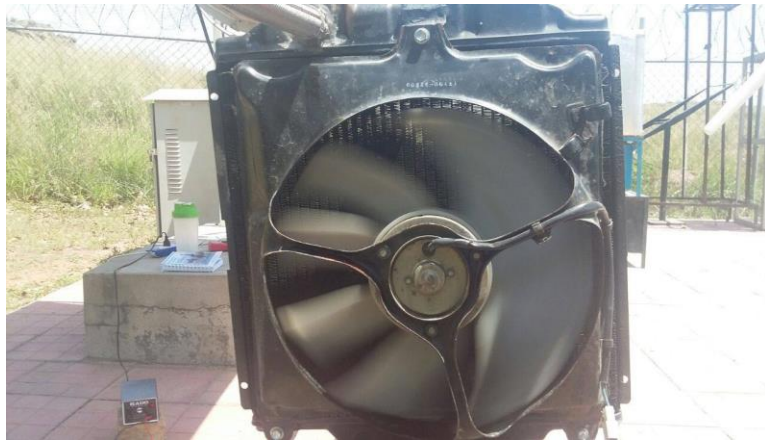
Figure3-4: Compact heat exchanger used. (Car radiator)
