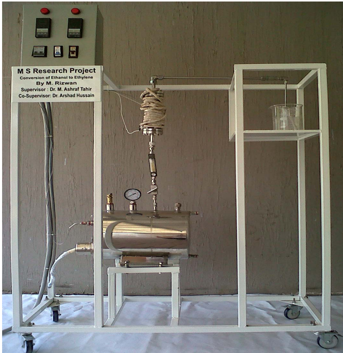
Figure 4.1: Experimental Rig for Dehydration of Ethanol.
