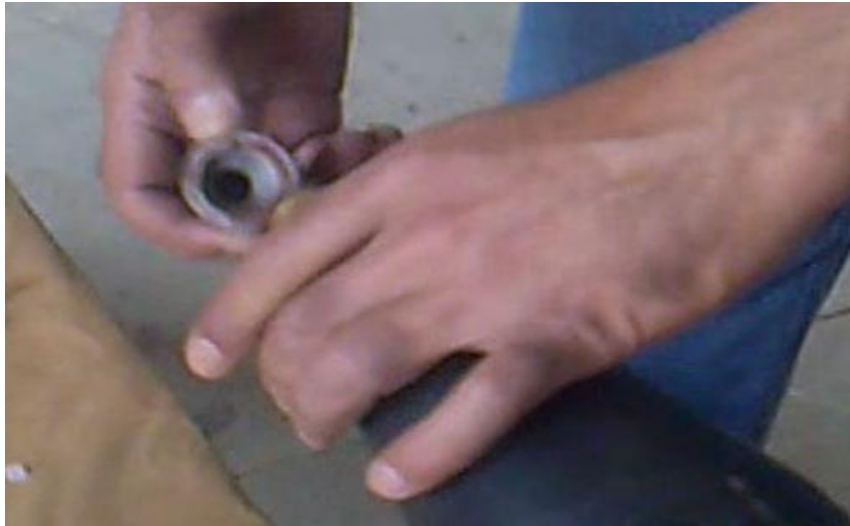
Figure: 5.5 Removal of Ogive head from 106 mm HEAT Round.
