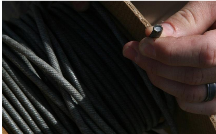
Figure: 2.5 Reinforced detonation cord filled with Pentaerythritol Tetranitrate (PETN).
