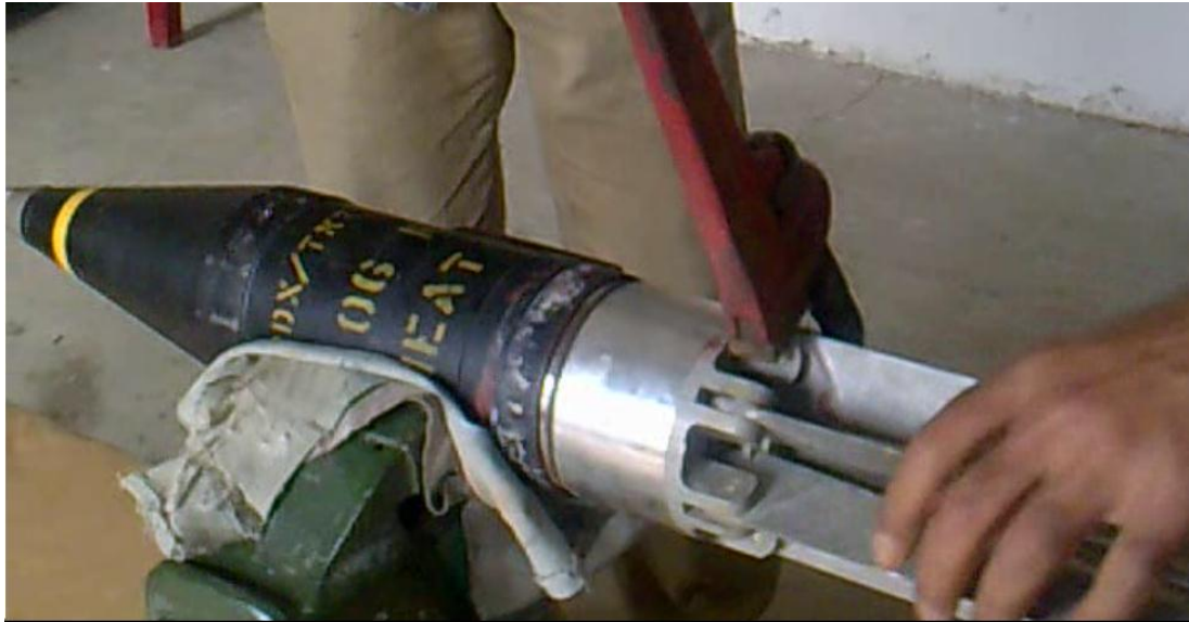
Figure: 5.1 Dismantling of 106 mm HEAT Round.
