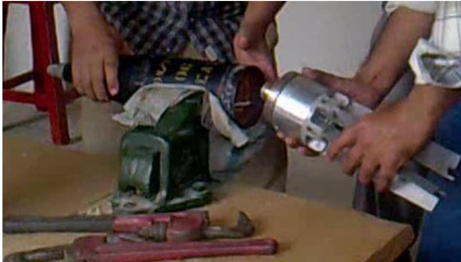
Figure: 5.3 Recovery of PIBD fuse with Fin Assembly from 106 mm HEAT Round.
