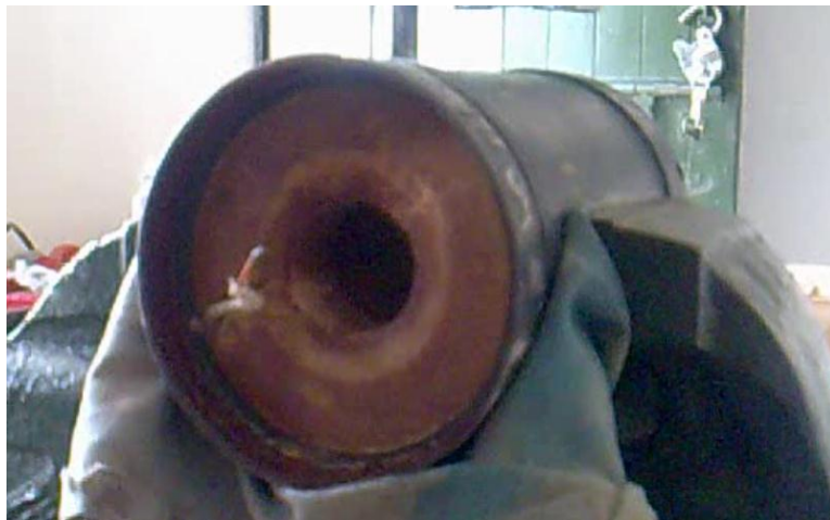
Figure: 5.4 106 mm HEAT Round filled with Composition B Explosive and Wire lead.
