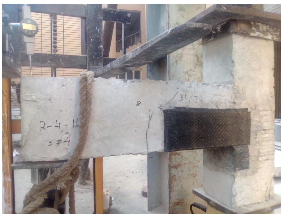
Figure 3.10: Collars Installed at Column Ends
