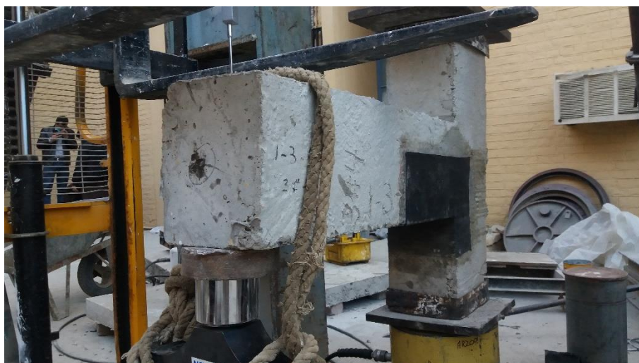
Figure 3.9: Placing of repaired specimen for test
