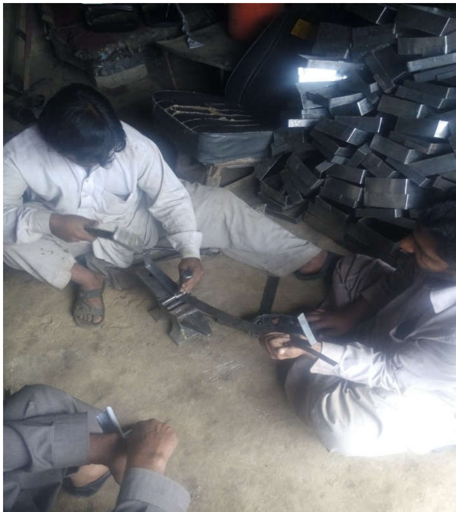
Figure 12: Bending of strips
