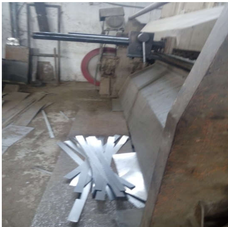
Figure 9: Fabrication of steel strips
