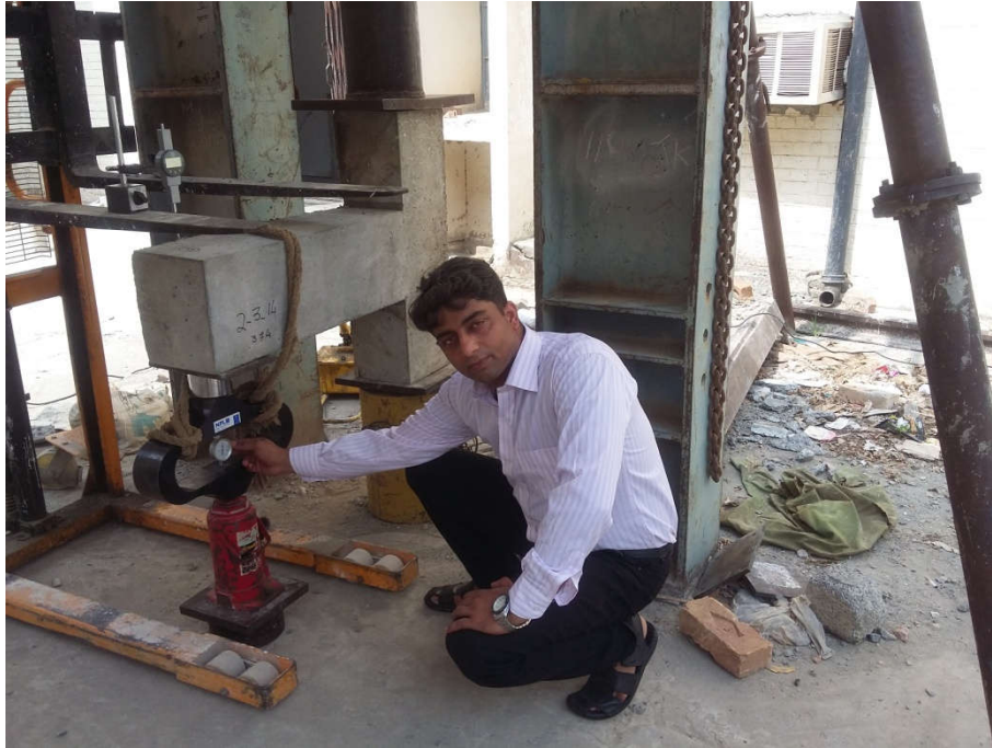
Figure 21: Placing of Specimen for Test
