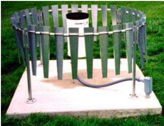
Figure 2.4. A wind shield placed around rain gauge to reduce wind effect.
