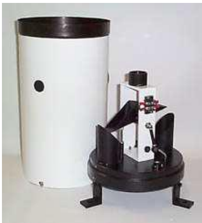
Figure 2.2. A tipping bucket rain showing the bucket tips and cylinder.
