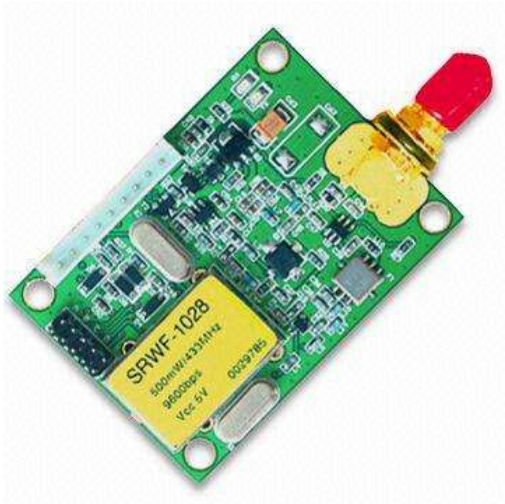
Figure 2. 5. Wireless transceiver of range (100-150) m.
