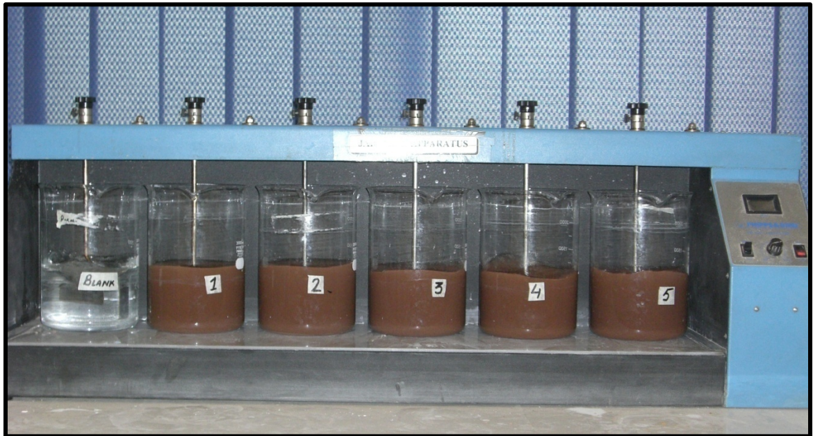
Figure 3.3 Jar testing apparatus (Phipps and Bird PB-700 TM -Virginia-USA)
